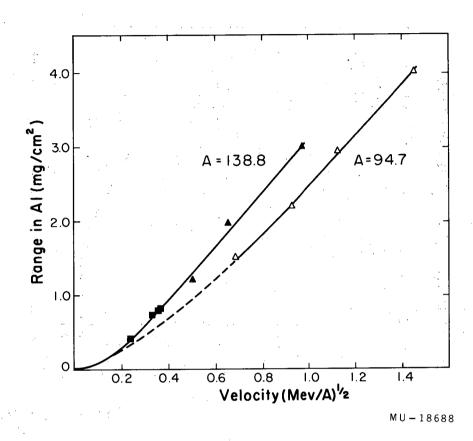
Fig. 6. Range-velocity curve in Al for the median light (open points) and heavy (closed points) fission products. The triangles are from the range measurements of this work and the energy measurements of reference 13. The squares are from the measured range of Tb<sup>149</sup> recoils (formed in nuclear reactions, reference 23) converted to the median heavy fragment of the same velocity.
