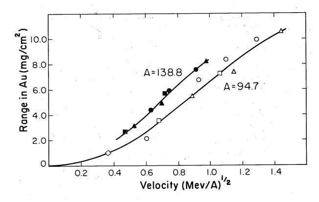
Fig. 8. Range-velocity curves in Au for the median light (open points) and heavy (closed points) fission products. The squares are from this work and Fig. 6, the triangles from reference 13, the circles from reference 14, and the diamond from reference 15 and Fig. 6.
