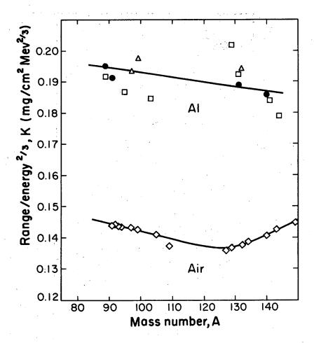
Fig. 14. The constant K in the relation  $R_i=K_i$   $E^{2/3}$ , calculated from the initial energy in Mev (reference 12) and the total range (in mg/cm<sup>2</sup>). Closed circles are from range data of this work, squares reference 16, triangles reference 15, diamonds reference 11.
