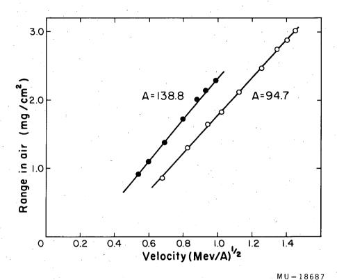
Fig. 7. Range-velocity curves in air for the median light (open points) and heavy (closed points) fission products. Total range measurements are from reference 11 and the energy measurements are from reference 14.
