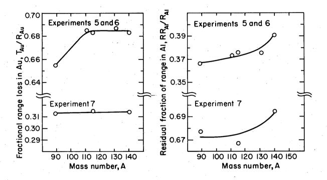
Fig. 11. Fractional range loss in Au  $(T_{Au}/R_{Au})$  and fractional residual range in Al  $(RR_{Al}/R_{Al})$ . If these two fractions sum to unity the range-energy curve in Al is proportional to the range-energy curve in Au, for the particular values of  $T_{Au}$  and  $RR_{Al}$ .
