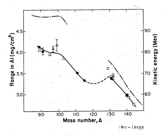
Fig. 4. Range in Al and kinetic energy of products from fission of U<sup>235</sup> induced by thermal neutron irradiation. The experimental range values are designated as follows: The circles from this work; The triangles from reference 15; and the squares from reference 16, normalized to these results by the factor 1.084. The dot-and-dash curve shows the kinetic energy of the products as taken from reference 12.
