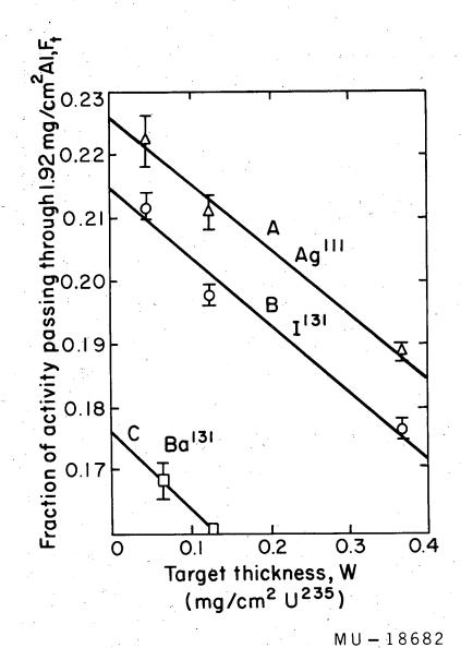
Fig. 3. Least-squares fit to linear dependence of  $F_t$  on W. The ratio  $(k_{Al}/k_W)$  of initial rate of velocity loss in the target to that in Al was determined for  $Ag^{111}$ ,  $I^{131}$ , and  $Ba^{140}$ . Aglil: kAl/kW Ilio: kAl/kW Ba : kAl/kW = 1.48 (least squares) = 1.45 (least squares) = 1.49
