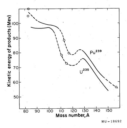
Fig. 15. The energy of the fission products. The solid curves are taken from reference 12. The circles were obtained from range measurements and extrapolated range-energy parameters.
