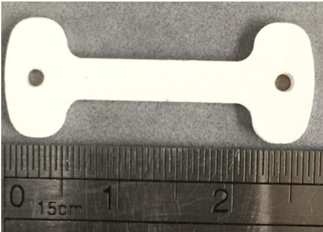
Figure 2.1: Example of dog-bone shaped ceramic green body after pressing
