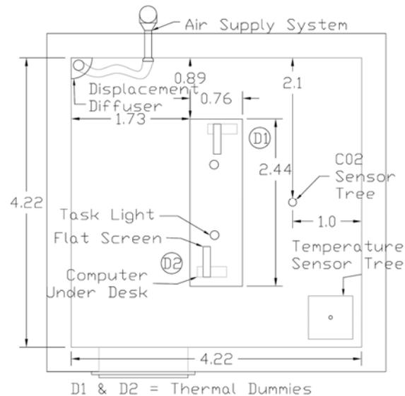
Figure 2. Layout of test chamber.
