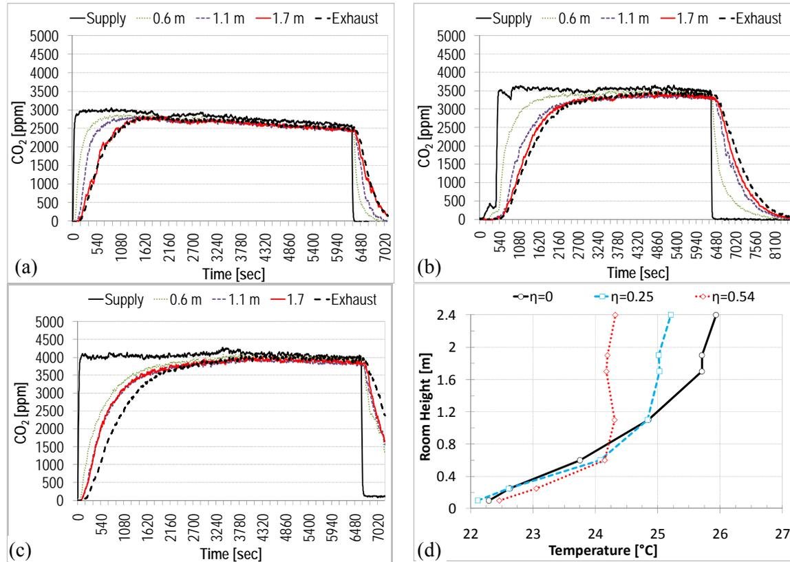
Figure 3. For (a) (b) and (c): CO<sub>2</sub> concentrations for the step-up method at the supply, exhaust and at 0.6, 1.1 and 1.7 m for: (a) test 1 where there is only DV; (b) test 2 where the radiant panels remove 25% of the load; and (c) test 3 where the radiant panels removed 54% of the load. (d) Air temperature profiles for the three tests described in Table 2.
