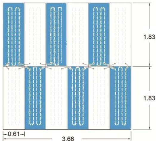
Figure 1. Active radiant panels (blue) configuration.
