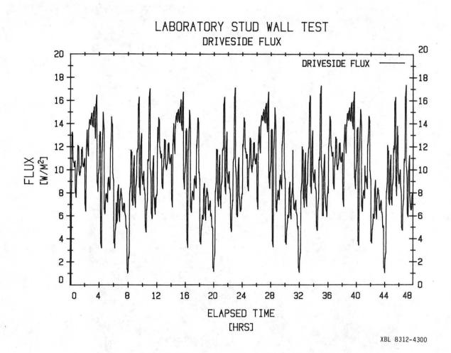
Figure 5. Driveside flux for laboratory test of insulated stud wall (fundamental frequency = one cycle every 12 hours).
