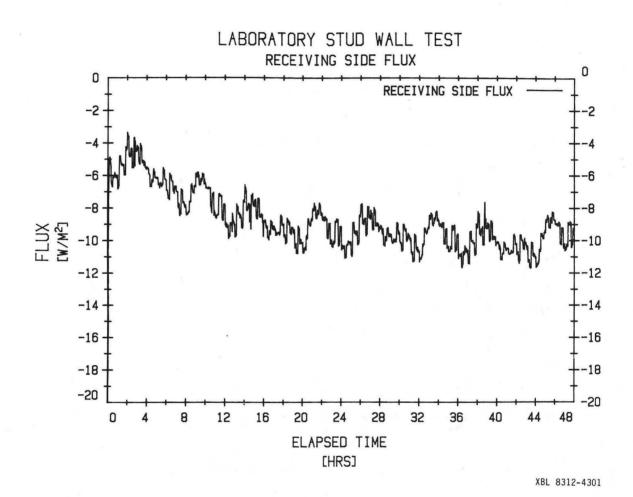
Figure 6. Receiving side flux for laboratory test of insulated stud wall.
