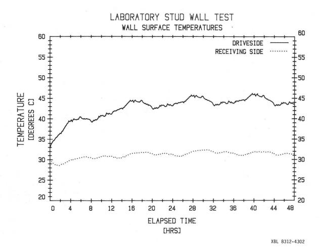
Figure 7. Driveside and receiving side temperatures for laboratory test of insulated stud wall (fundamental frequency = one cycle every 12 hours).
