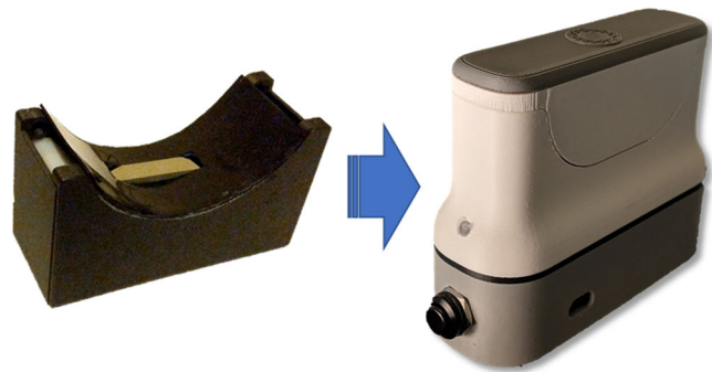
Fig. 6 Evolution of the non-invasive optical device from the exploratory prototype phase to the current production-ready phase. The exploratory and prototype phase devices collected two optical data points whereas the current product collects four optical data points, thus potentially improving the specificity of detection.
