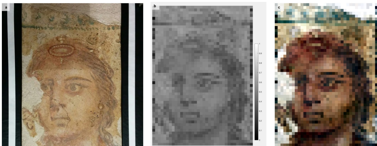
Figure 5.10: (a) An RGB image of the face of a figurative painting recovered from Tomb 3510. (b) The 3D matrix constructed in Matlab from the individual spectra collected in the scan. (c) The extracted image from the final reconstructed 3D data cube in ENVI.
