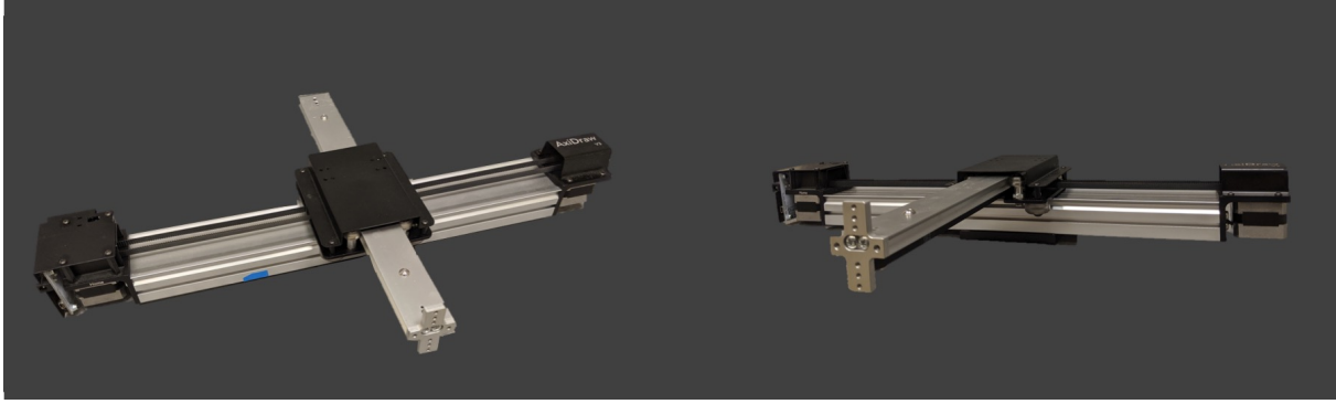
Figure 5.4: The Axidraw V3, a pen-plotting instrument customized for novel x - y scanning operation to drive the FO cable over the surfaces of paintings.
