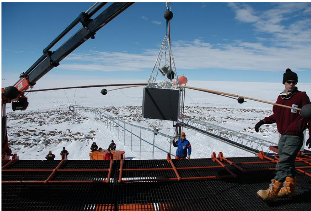
Figure 2.1: A photo of a MINIS payload being transferred to the flight line. The electric field booms are clearly visible as well as the ground planes surrounding the payload.
