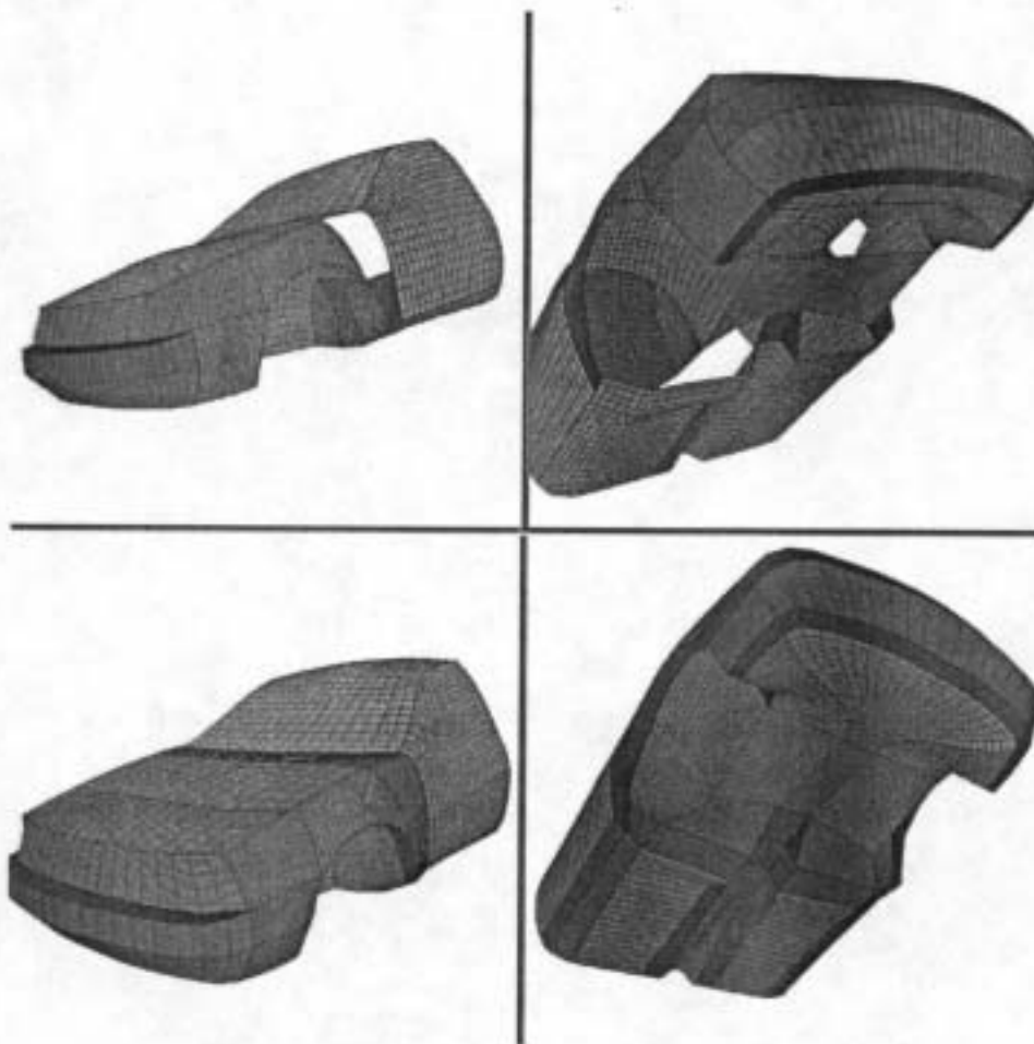
Figure 3.13: Car body with “holes” ( top ) and its approximation ( bottom ).
