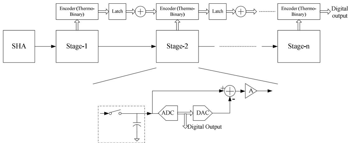
Figure 3.3 Detailed Pipeline ADC Architecture.
