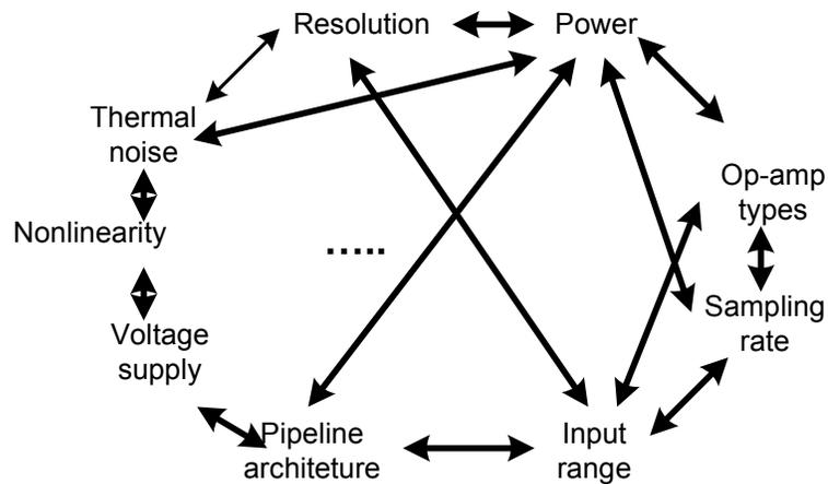
Figure 3.4 Pipeline ADC Design Matrix.
