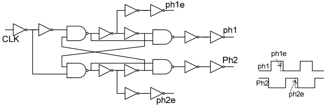
Figure 5.2 Non-overlapping Clock Generator.
