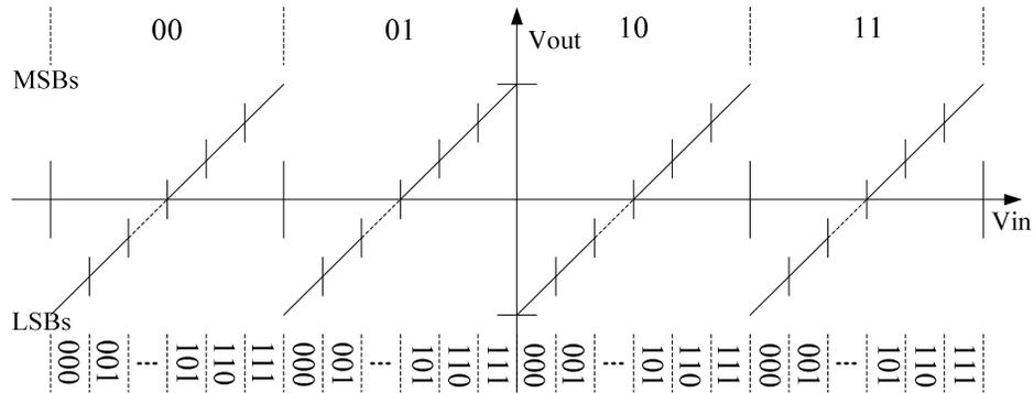
Figure 3.1 Pipeline ADC Transfer Curve.
