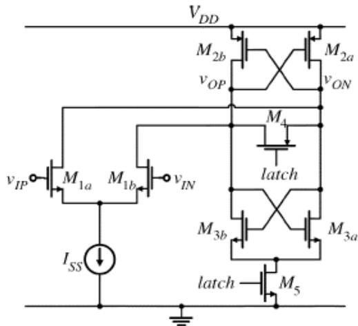
Figure 3.11 Class-AB Latched Comparator.
