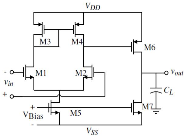
Figure 3.7 Amplifier-type Comparator.
