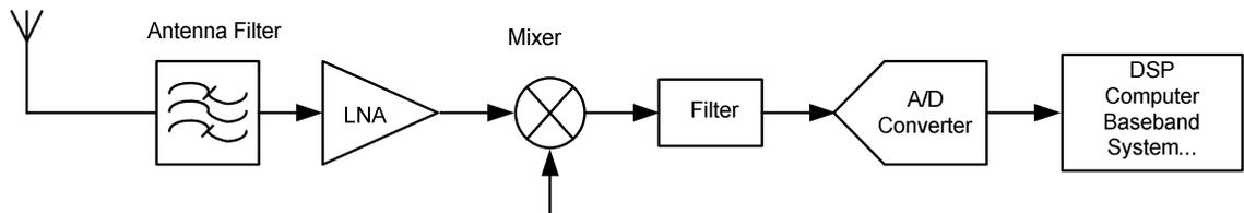
Figure 1.1 ADC in the Interface between Analog and Digital World.
