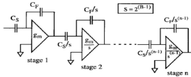
Figure 4.3 Capacitor Scaling Down.
