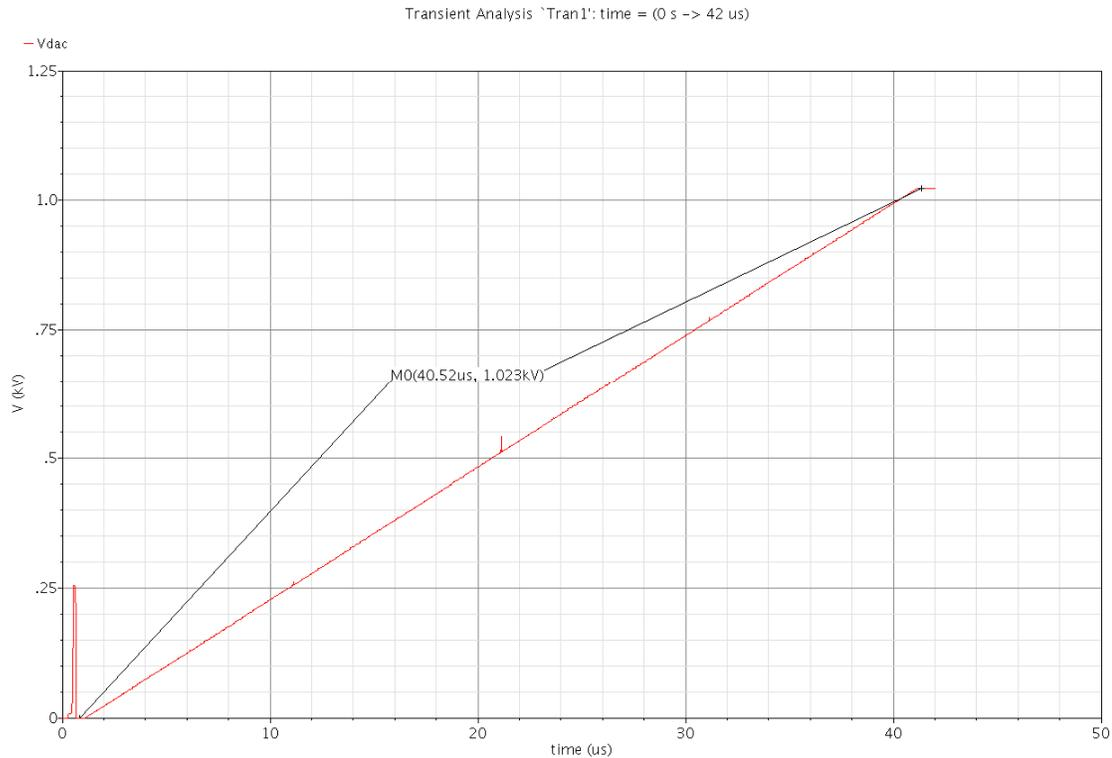
Figure 5.11 Ramp Signal to Verify Monotonicity.
