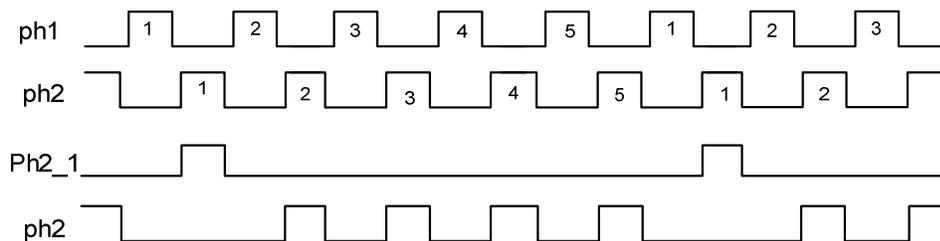
Figure 5.8 Phase Scheme of Cyclic ADC.
