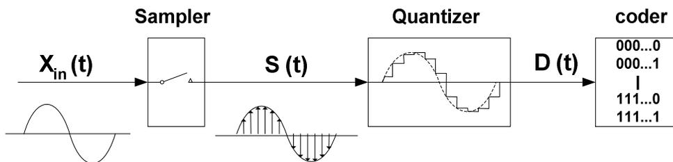
Figure 1.3 Analog-to-Digital Converter Block Diagram.
