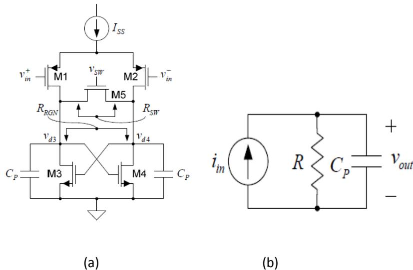
Figure 3.8 (a) Typical Latch-type Comparator (b) Equivalent Small Signal Model.
