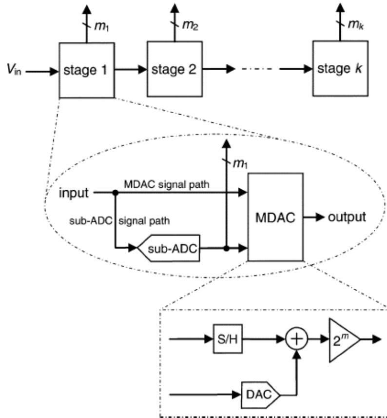
Figure 2.4 A Pipelined ADC.
