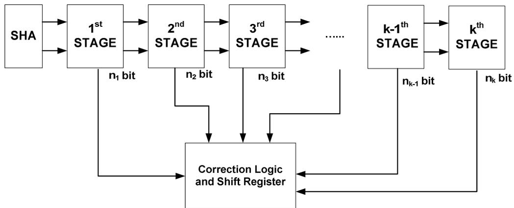
Figure 4.8 Pipeline ADC Structures.
