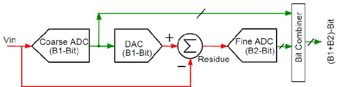
Figure 2.2 Two-Step Flash ADC.
