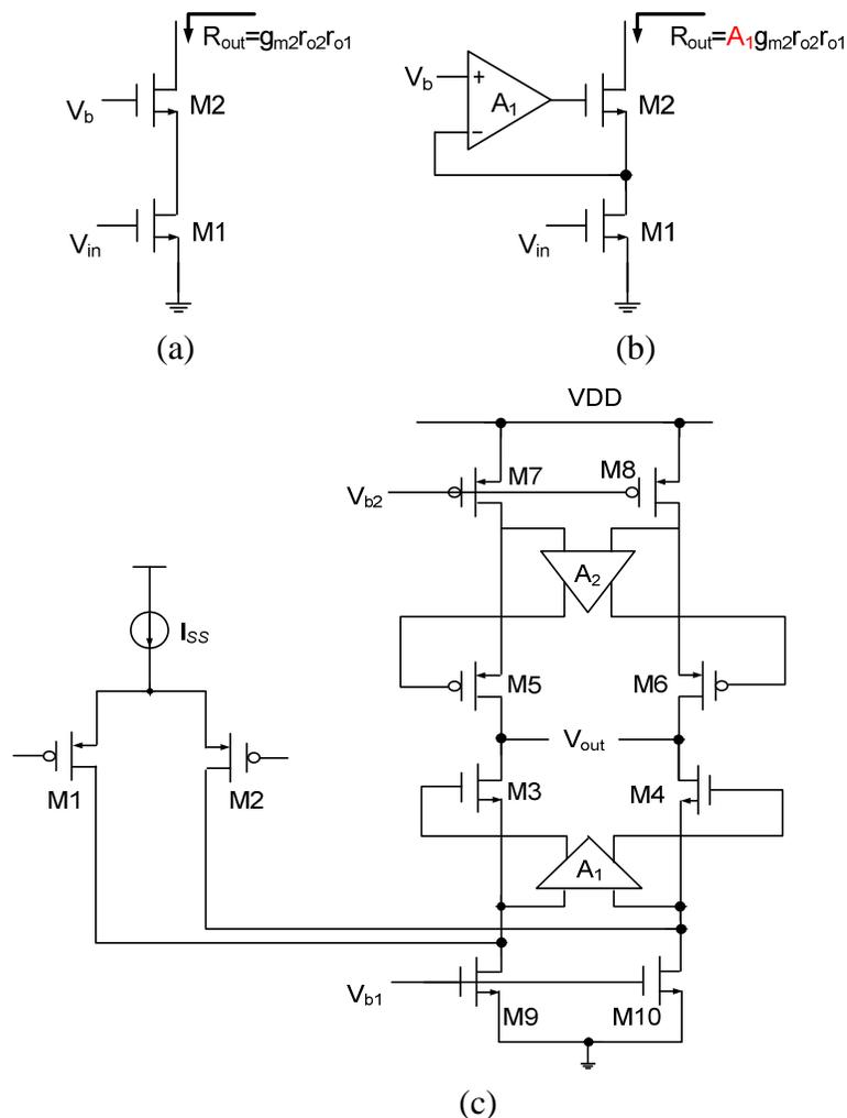
Figure 3.18(a, b) Gain Boosting Technology, (c) Folded-cascode Op-amp with Gain Boosting.
