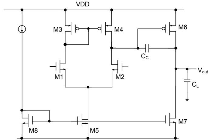
Figure 3.15 Two-stage Op-amps.
