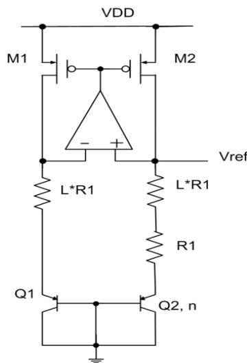
Figure 3.22 Bandgap Voltage Reference.
