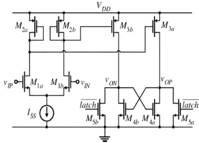
Figure 3.10 Static Latched Comparator.
