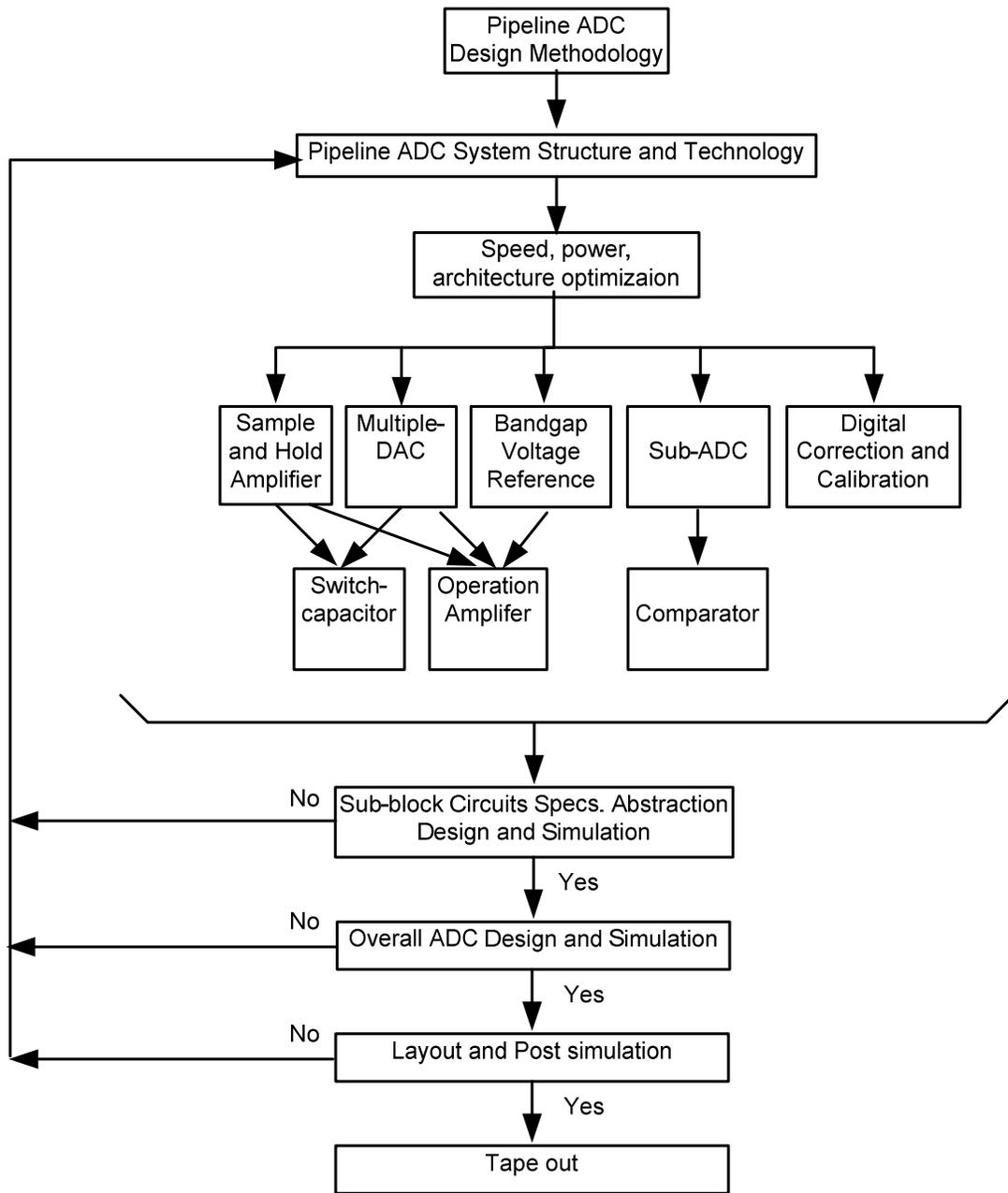
Figure 3.5 Pipeline ADC Design Flow.
