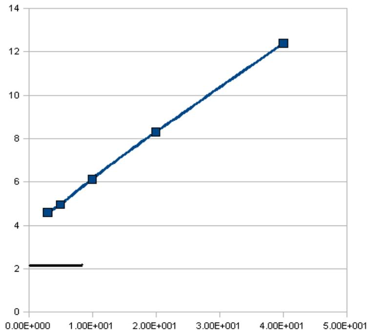
Figure 5.10 Total Power Consumption vs. Sampling Frequency.
