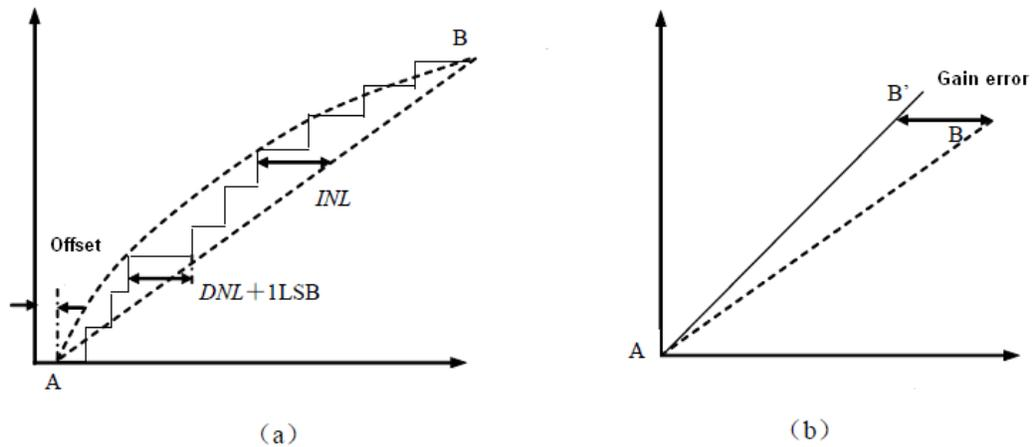
Figure 1.4 ADC Static Errors.
