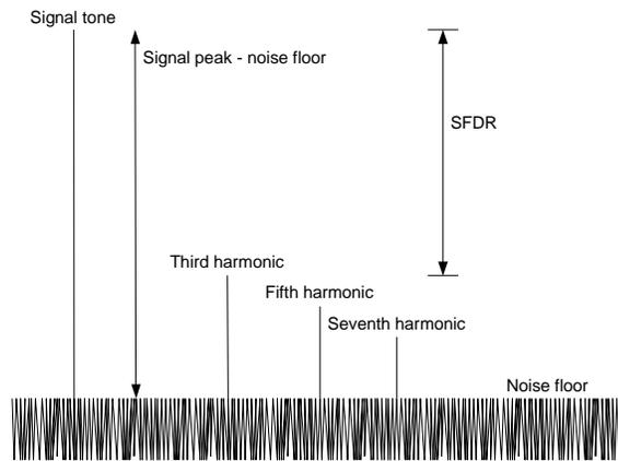
Figure 1.5 ADC Dynamic Parameters.
