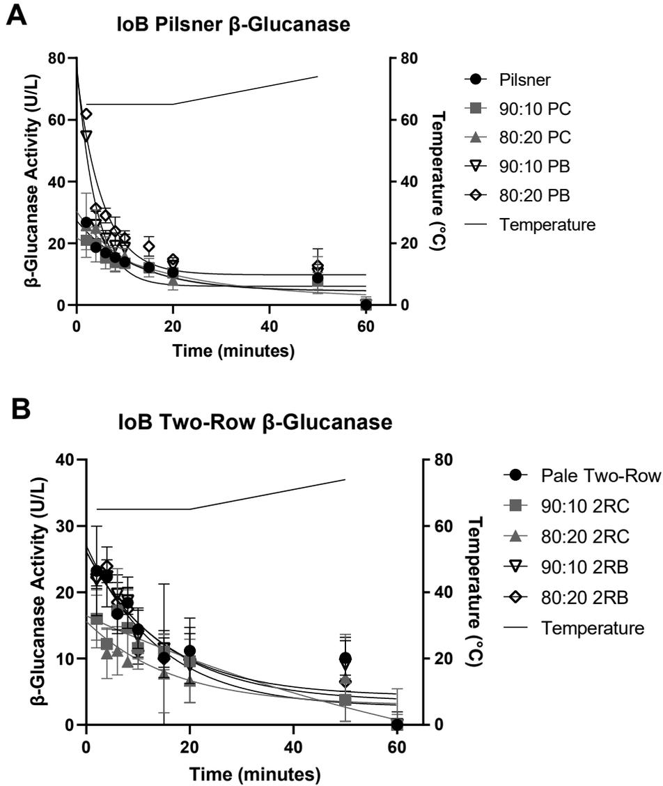
Figure 3.4:  $\beta$ -glucanase throughout the temperature progression of the IoB mash for (A) Pilsner malt and (B) two-row pale malt. Error bars represent one standard deviation. PC is Pilsner malt and caramel malt blend, PB is Pilsner malt and barley blend, 2RC is two-row pale malt and caramel malt blend, and 2RB is two-row pale malt and barley blend.
