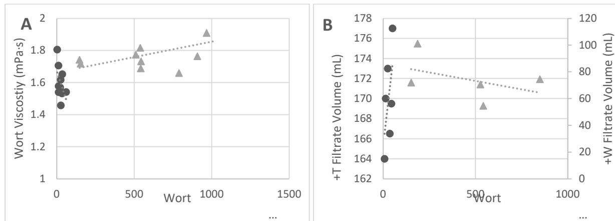
**Figure 4.3:** (A) Wort viscosity plotted against wort  $\beta$ -glucan content. (B) Wort filtrate volume after 25 minutes plotted against wort  $\beta$ -glucan content for mashes with  $\beta$ -glucanase from *Trichoderma* (●) plotted on the primary y-axis and wild barley (▲) plotted on the secondary y-axis.
