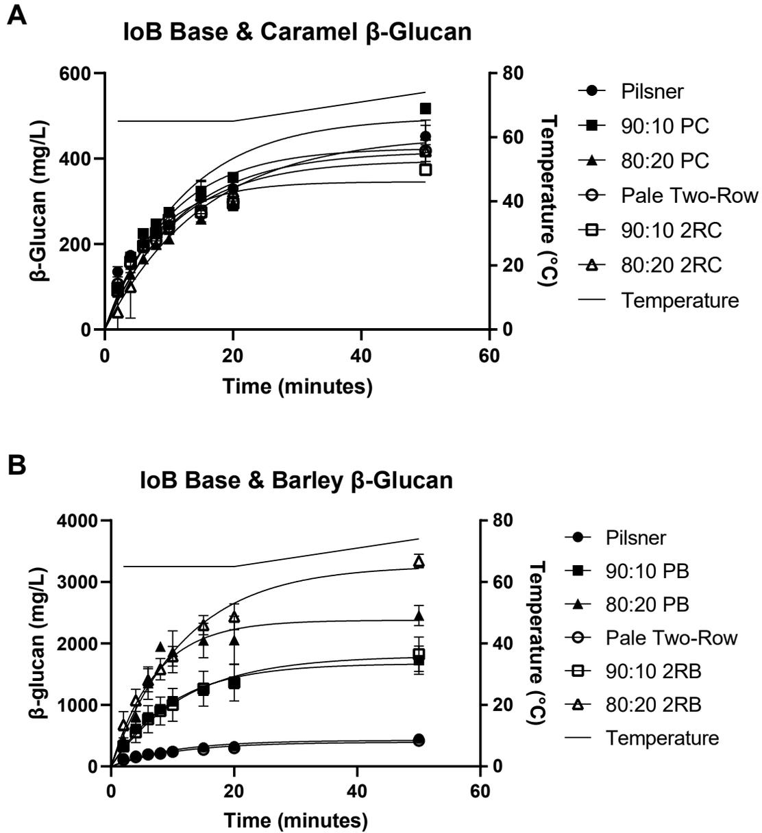
Figure 3.5:  $\beta$ -glucan concentration over the temperature progression of the IoB mash for base malt in comparison and combined with (A) caramel malt and (B) barley. Error bars represent one standard deviation. PC is Pilsner malt and caramel malt blend, PB is Pilsner malt and barley blend, 2RC is two-row pale malt and caramel malt blend, and 2RB is two-row pale malt and barley blend.
