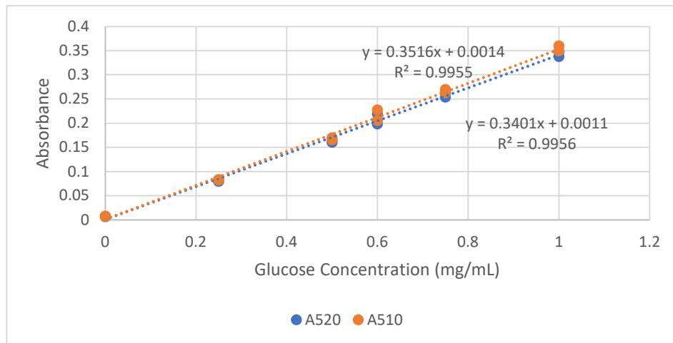
Figure 2.5: Glucose standard curves measured by the spectrophotometer at absorption wavelengths of 520 nm (A520) and 510 nm (A510). Correlation constants and equations for the lines of best fit are displayed on the chart.
