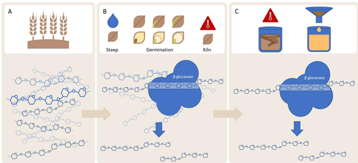
*Figure 1.1:* A visual description of the progression from barley (A) to malt (B) to wort (C) and how  $\beta$ -glucan is synthesized then hydrolyzed to progressively lower levels by  $\beta$ -glucanase.
