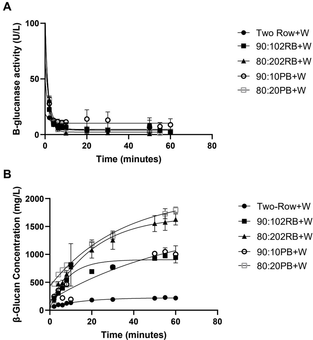
Figure 4.2:  $\beta$ -glucanase activity (A) and  $\beta$ -glucan content (B) over time during loB mash with thermostable  $\beta$ -glucanase from wild barley added (+W). Results displayed are for Pilsner and pale two-row malts in combination with 10% and 20% barley. Error bars represent one standard deviation from the mean.
