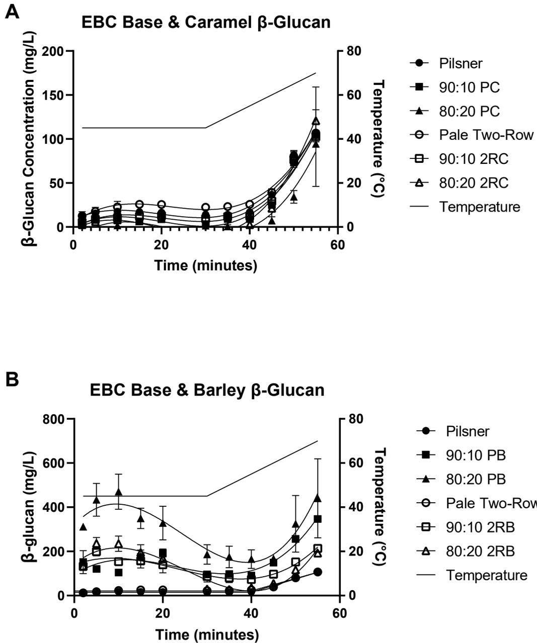
Figure 3.3:  $\beta$ -glucan concentration over the temperature progression of the EBC mash for base malt in comparison and combined with (A) caramel malt and (B) barley. Error bars represent one standard deviation. PC is Pilsner malt and caramel malt blend, PB is Pilsner malt and barley blend, 2RC is two-row pale malt and caramel malt blend, and 2RB is two-row pale malt and barley blend.
