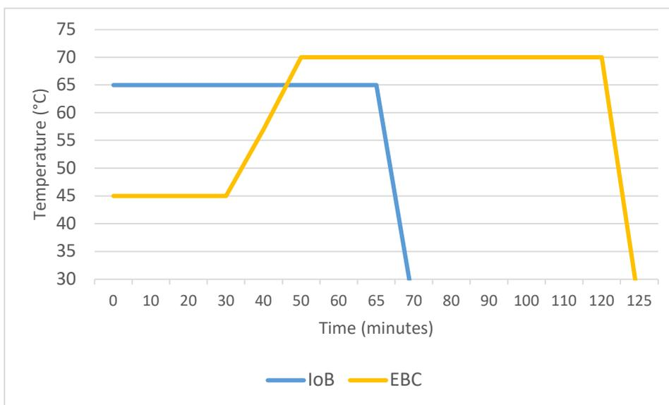
Figure 1.4: Temperature profile of the modified loB and EBC methods’ programmed temperature progression over the duration of the mash (6,29).
