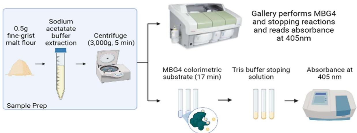
Figure 2.1: A graphic description of the analysis of  $\beta$ -glucanase with the manual method and with the Gallery autoanalyzer.
