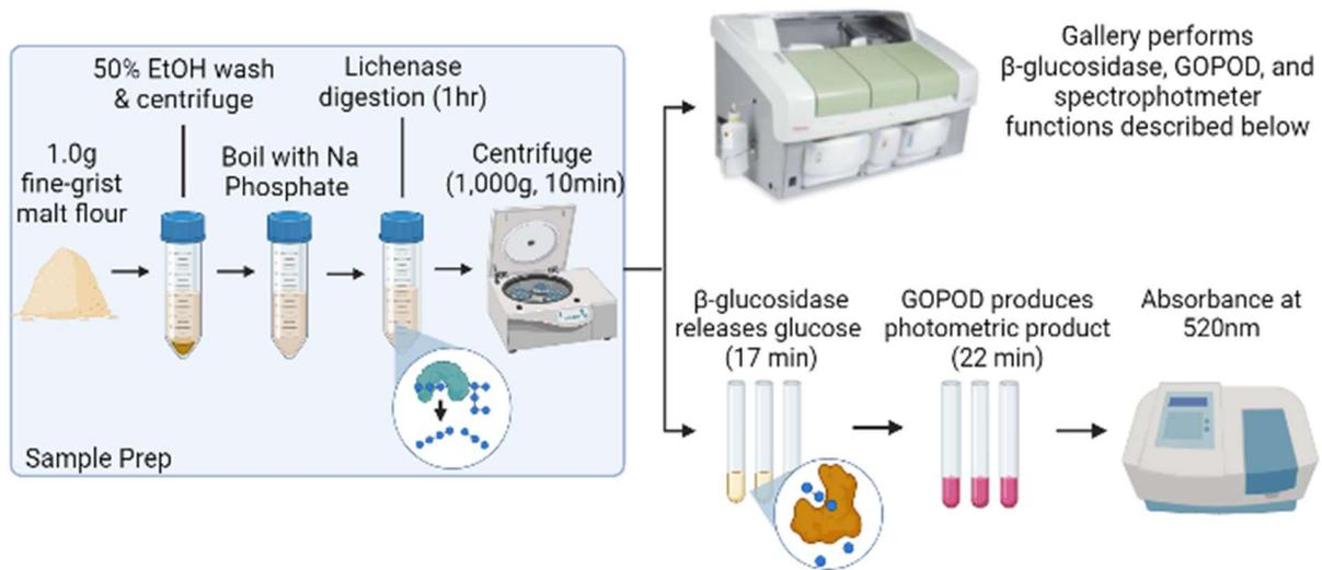
*Figure 2.2:* A graphical description of the manual enzymatic  $\beta$ -glucan method compared with the Gallery adapted method.
