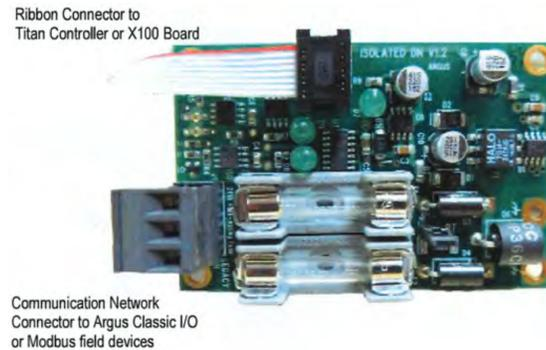
Figure 4.2: Argus Isolated Device Network Board (ISODN). The ribbon cable connects the ISODN with the Argus control panel. The screw terminal connects the ISODN with the BBB via a USB to RS-485 cable. Image retrieved from [9].
