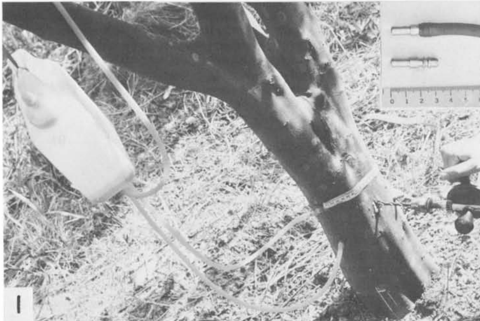
Fig. 1. Transfusion apparatus consisting of a 2-liter plastic reservoir, 7 mm rubber tubes and aluminum tube connector with dimensions of 6 \times 13 + 8 \times 5 + 7 = 13 (upper right). Manual drill was used for making three holes in the trunk.
