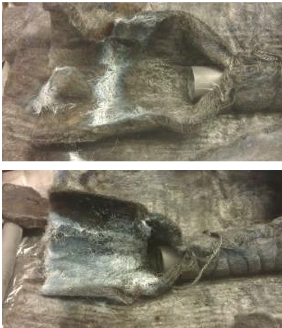
Figure 6.9: Photographs of BNNTs deposited the downstream end of the graphite tube.
