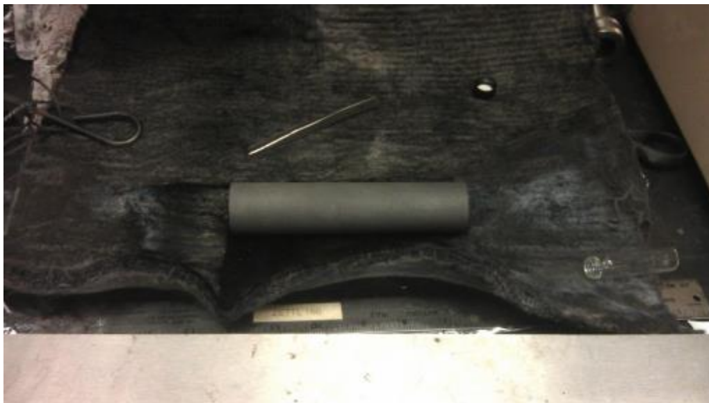
Figure 6.7: Photograph of graphite cylinder with insulation used for BNNT synthesis.
