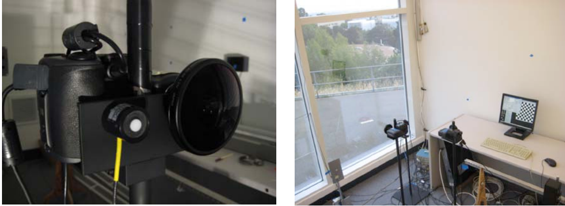
Figure 9: Typical Nikon990 setup for LDR image acquisition with adjacent vertical illuminance sensor (left). View of test room showing window-facing and VDT-facing camera orientation (right).
