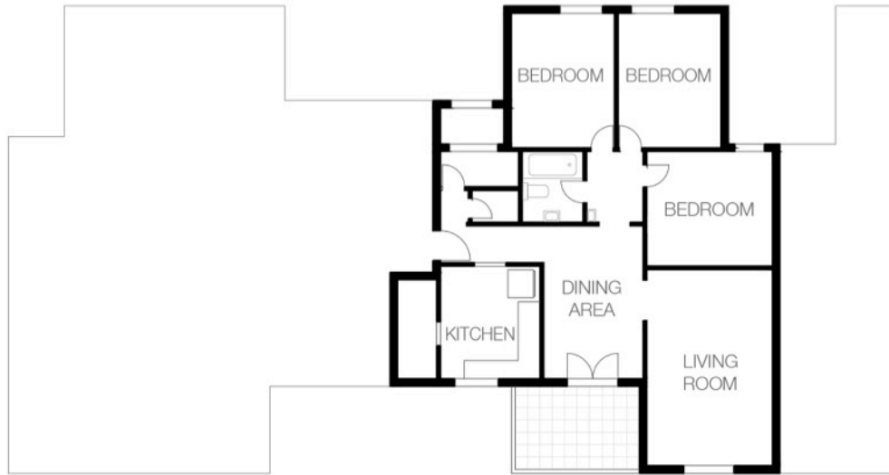
Figure 4.18 Typical residential unit with a living room closed off from the rest of the house. Beitar Illit, Hill A, Ya'ar Architects, ca. 1989. Schematic plan drawn by author. Author's drawing based on original plan available at The City Planning Division of Beitar Illit.
