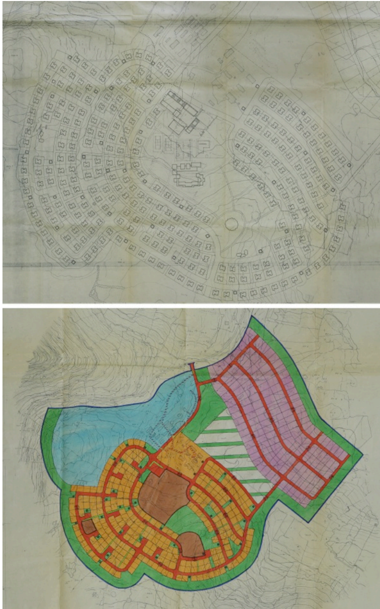
Figure 2.12 In January, 1978, Levitt shared his master plan with Settlement Department officials. Levitt arranged all private plots (painted in orange) around a civic center (in brown). In all, there were some 276 private plots, and an industrial area at the top-right corner (in purple) that was divided into 145 plots. Levitt allocated a large plot for agriculture (marked with slanted green lines) between the residential and industrial areas. Not everyone wanted these agricultural fields. Many settlers thought it was wasteful. But Etzion, who spent a few years in a kibbutz as a kid, insisted on having agriculture. 110 Eventually, he succeeded convincing his fellow activists that some agriculture would render their stay in Ofra more permanent.
