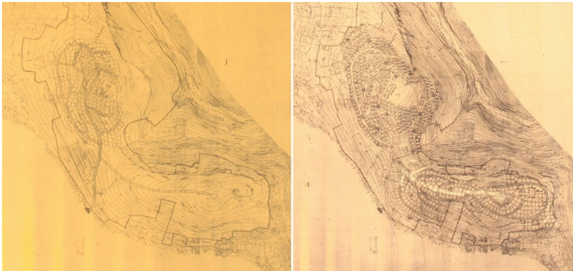
Figure 3.7 Plan drawings of Beit Arye from 1981 (left) and 1984 (right). Arranged around two separate public centers, all plots were uniformed in size. At one point, one of the future residents proposed enlarging
