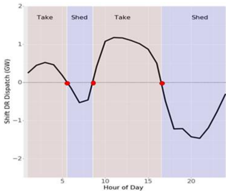
Figure 1-4. An idealized daily dispatch signal to which Shift resources would respond. Positive values of the dispatch indicate the need for resources to take load; negative values request a shed. To estimate the Shift resource, the DR-PATH model identifies loads that could be shifted within multi-hour windows centered on the zero points (red dots).
