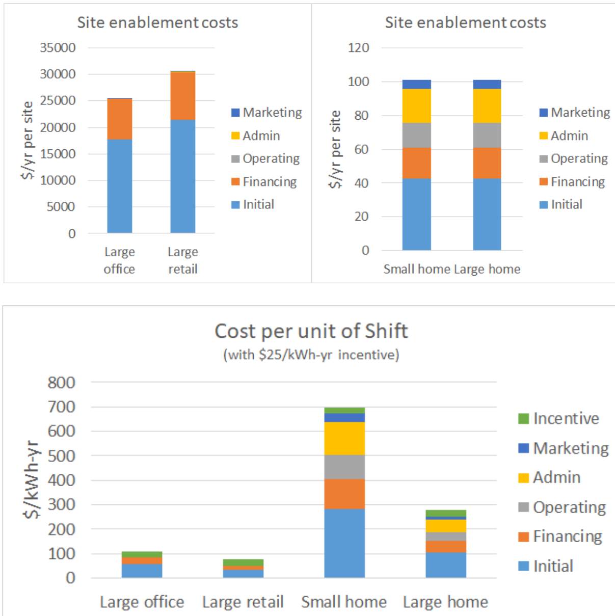
Figure C-2. Example site-level cost calculations for enabling different sites to perform Shift (top panels) and total resource costs for the Shift obtained at each site (bottom panel).
