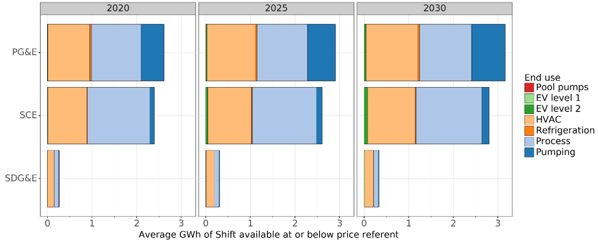
Figure 3-6. The Shift resource available at the BTM battery price referent (gray dotted lines in Figure 3-3), disaggregated by utility and end use. 37
