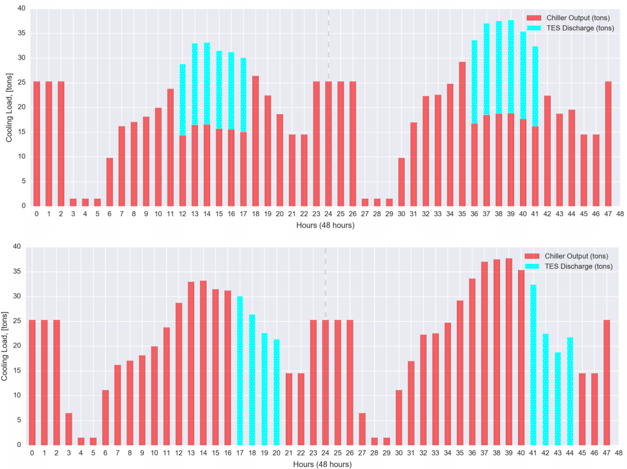
Figure D-2. Modeled TES system operation for a typical system under strategies to reduce mid-day peak load (top) and shift evening load (bottom). A system that is sized for the common peak-shaving strategy shown at top is able to shed 100 percent of evening load in a Shift scenario.
