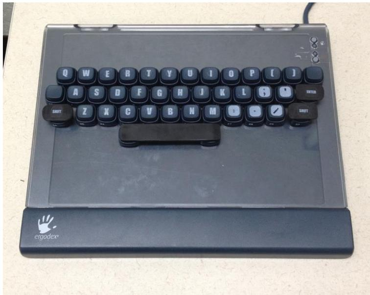
Figure 2. Keyboard with 19x19 mm key spacing.
