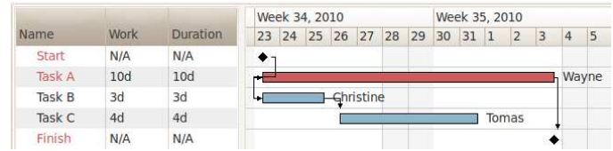
Figure 14: Gantt chart for Figure 13. Each Task has a single, dedicated staff. The critical path (light red) is Task A. We can ignore Saturday and Sunday (28th and 29th).
