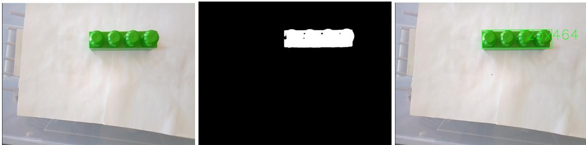
**Figure 2.1:** The three stages of image processing pipeline performed on a sample cuboid object. The left image shows the original image taken from the eye-in-hand camera. The center image shows the HSV segmented image. The right image shows the detected blob with a rectangle representing the centroid, dimensions and angle of the major and minor axes.
