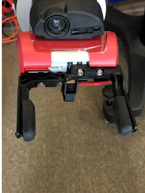
**Figure 1.2:** The Baxter's parallel gripper with eye-in-hand camera and IR sensor
