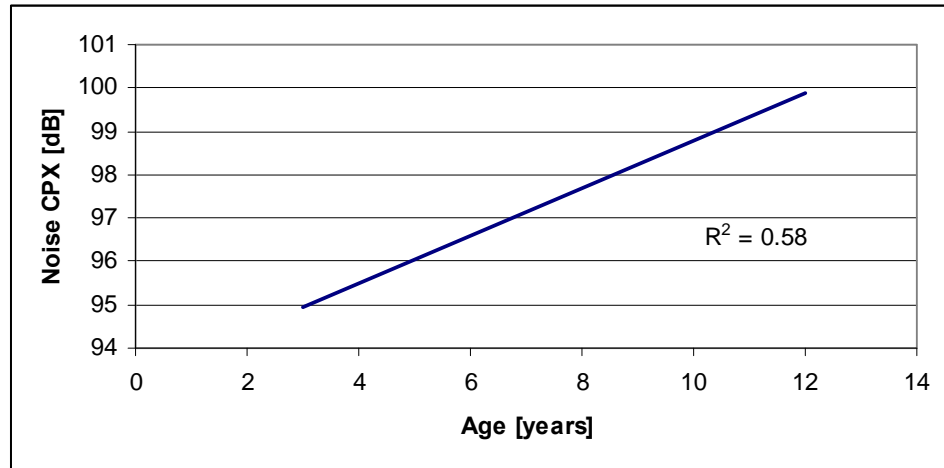
Figure 1.3. Results of CPX noise measurements in Arizona on Asphalt-Rubber Friction Course at different ages [20] performed at 96 km/h (60 mph) [20].
