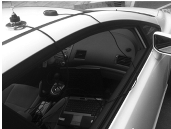
Figure 2.2 Node setup on a vehicle
