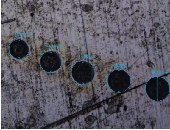
(a) Crater diameters measured for different lens positions.
