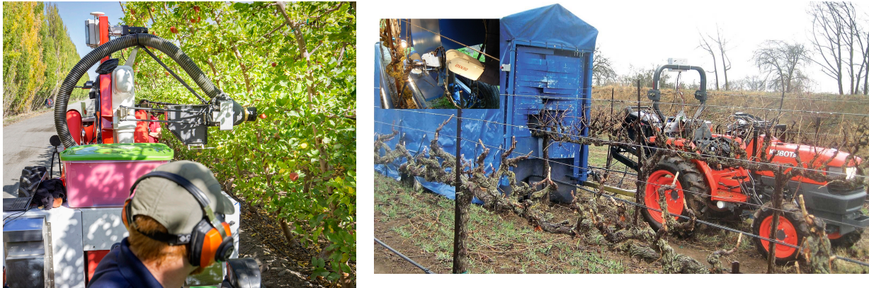
Figure 2 a) Lettuce thinning robotic implement (Blue River – NSF photo archive); b) Robotic mechanical weeder (courtesy of Steve Fennimore); c) Operators of an Abundant Robotics automated vacuum harvester monitor the test vehicle working a Fuji apple block during the 2016 Washington apple harvest. (TJ Mullinax/Good Fruit Grower); d) Robotic vine pruner (Vision Robotics).
