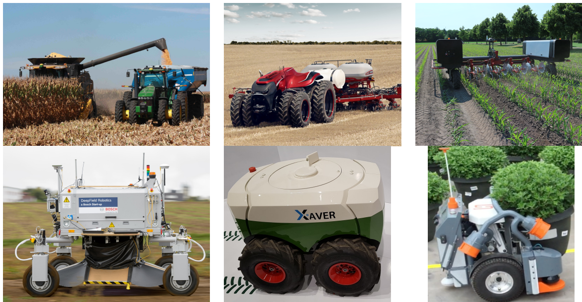
Figure 1 a) Auto-steered harvester and fully autonomous tractor pulling a grain cart for harvester unloading (Photo courtesy of Kinze Manufacturing/PrecisionAg.com); b) Cabinless fully autonomous general purpose tractor (CASE IH) and c) Robotti - AGROINTELLI, Denmark; d) Bonirob-Picture: Bosch; e) Autonomous robot seeder (Fendt - AGCO GmbH); f) Nursery robot for moving containers (Harvest Automation, USA).
