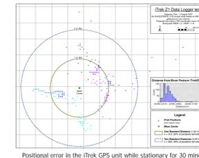
Positional error in the iTrek GPS unit while stationary for 30 minutes.
