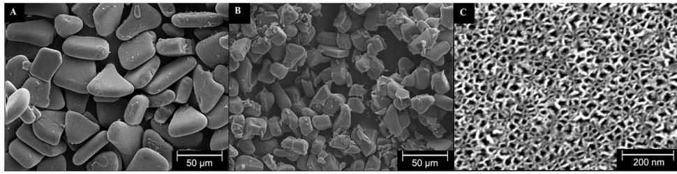
**Figure 1.** Scanning electron microscope (SEM) images of the two different pSiO<sub>2</sub> microparticle sizes used in this study: (A) pSiO<sub>2</sub>\_21/40 and (B) pSiO<sub>2</sub>\_6/20. (C) Plan-view image of the pore structure on the (100) surface of the particles.
