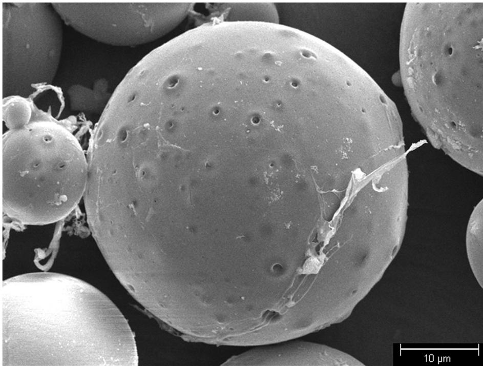
**Figure 5.** SEM image of PLGA-pSiO<sub>2</sub>\_21/40-DNR microspheres, showing the presence of micron-scale voids at the surface of the microspheres.
