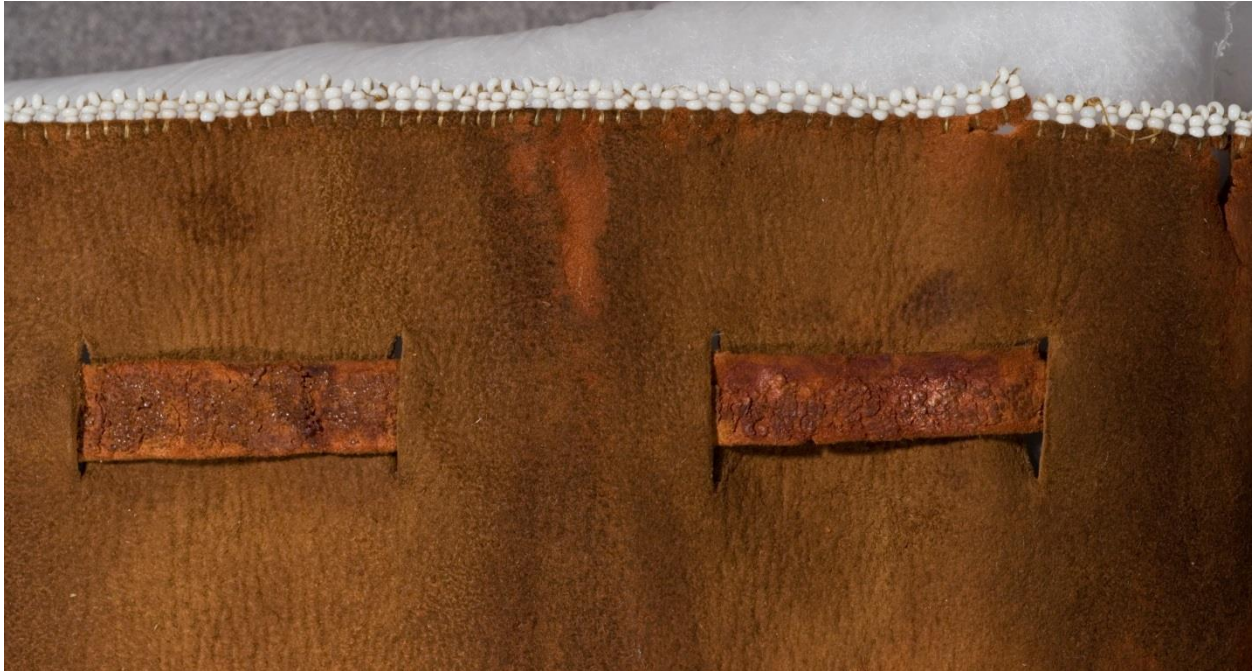
Figure 28: After treatment, detail of the strap where darkening occurred during the application of consolidant.
