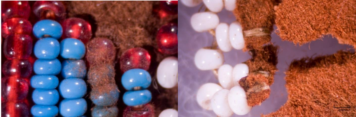
Figures 11 & 12: Before treatment, photomicrographs of the beads covered in powder from the leather (Left). Before treatment, photomicrograph of a tear along the opening of the bag that is creating an instability for the beaded element (right).
