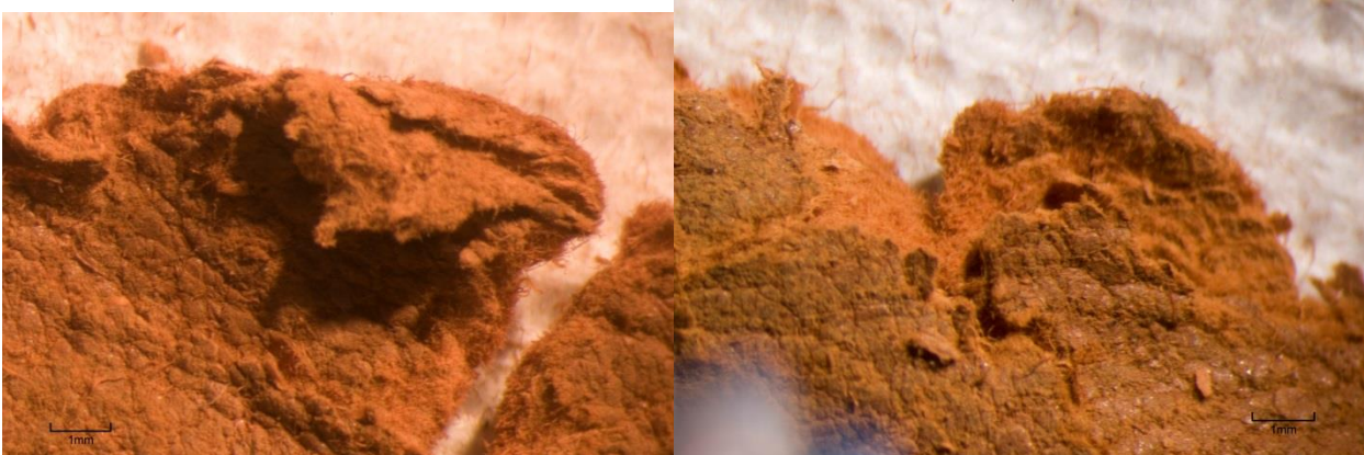
Figures 15 & 16: Before treatment, photomicrographs of the delaminating leather along the structural tear.
