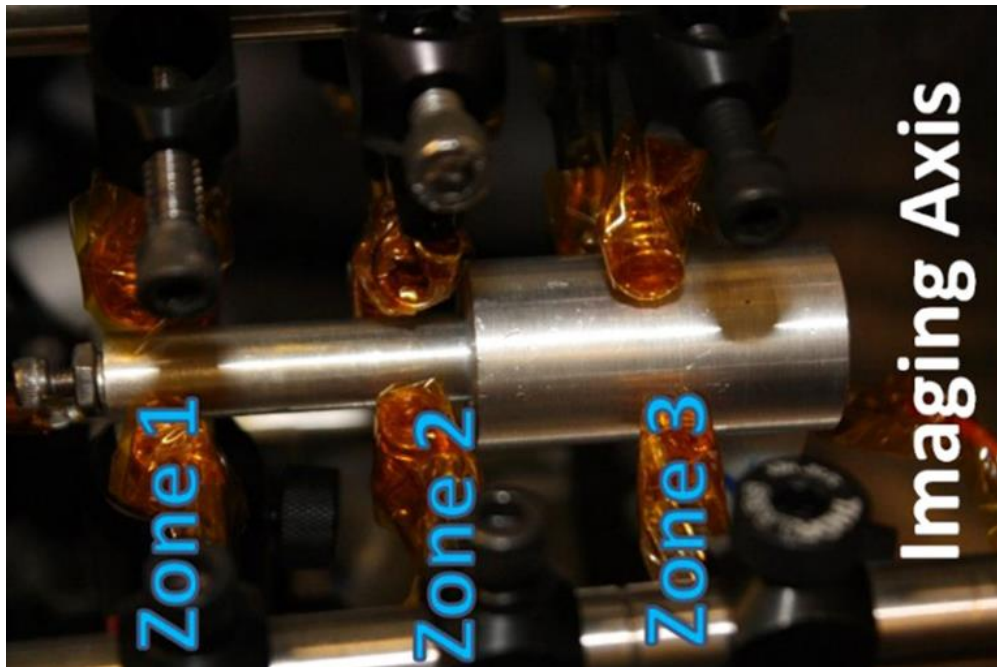
Figure 26: Coaxial gap experiment with b-dot array zones labeled.
