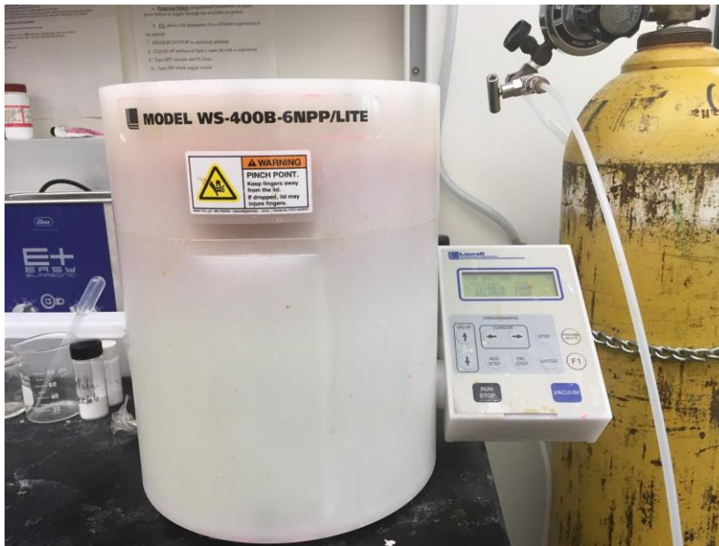
Figure 2- 15: The spin coater was used in this experiment to deposit a uniform thin film on a flat substrate with a specific thickness. This device also was used for drying substrates.
