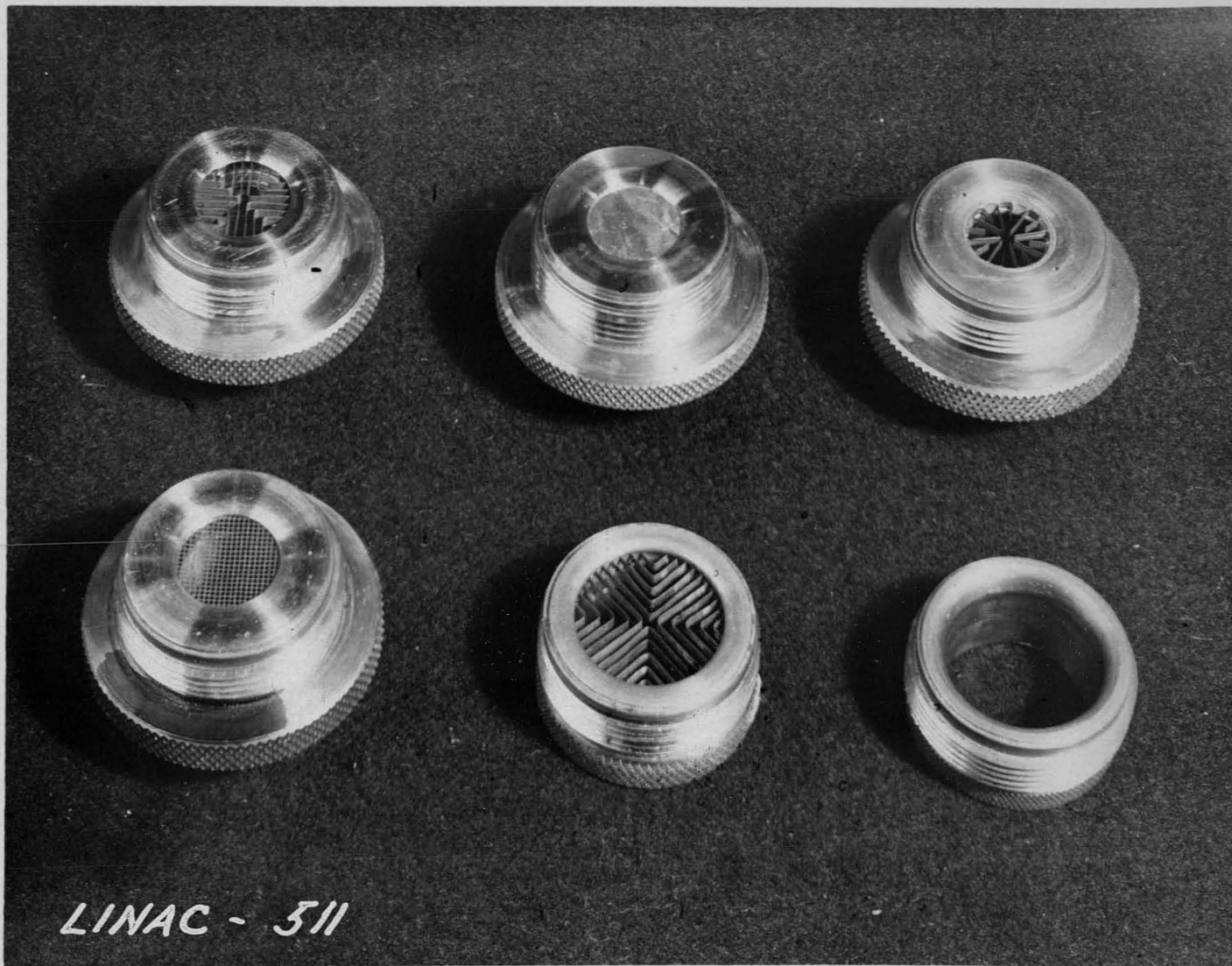
PHOTOGRAPH OF VARIOUS TYPES OF SLAT GRIDS AND BERYLLIUM FOILS MOUNTED IN HOLDERS
