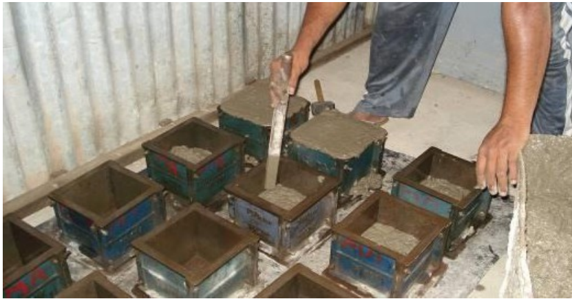
Figure 2: Concrete cubes for testing Error
