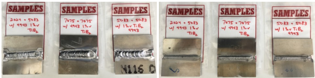
Figure 4.2.a Initial welding samples with small plates
