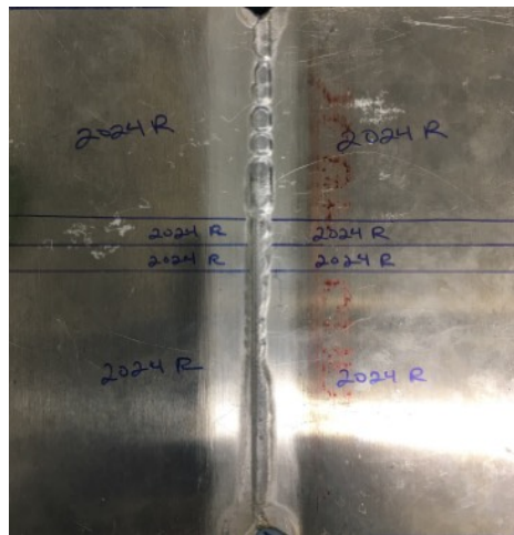
Figure 3.3 Cut Lines Along 2024 & 2024 Weld Length
