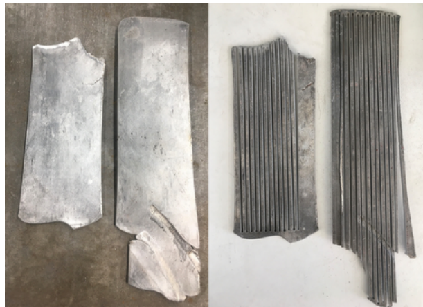
Figure 3.1.b 4943 1.25%v TiB 2 Filler (a) after hot rolling and (b) after water jet cutting
