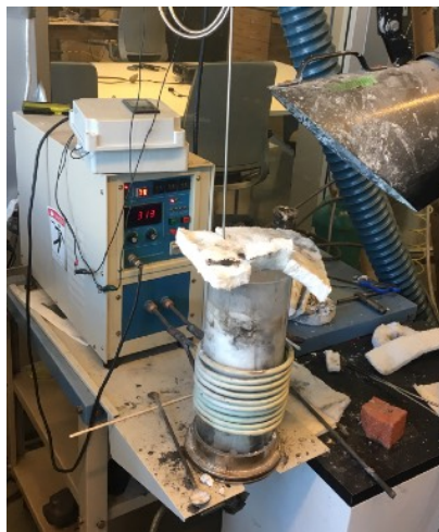
Figure 3.1.a Furnace for Alloying 4943 Nanocomposite Filler Material
