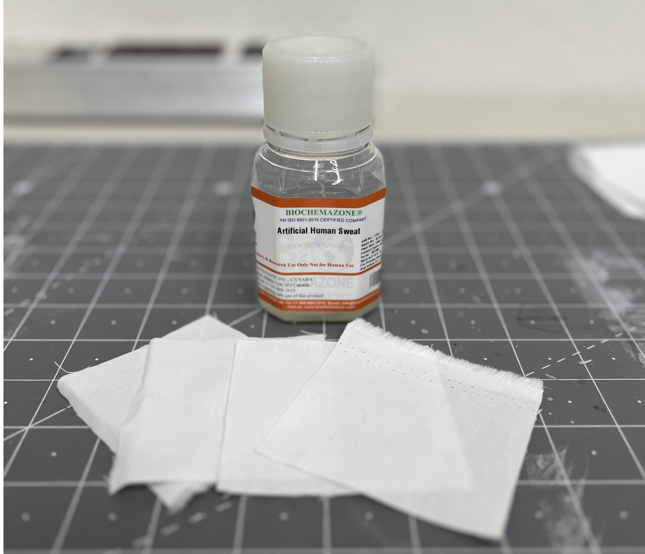
Figure 6.3: 100% cotton swatches and synthetic perspiration used in verification trials.
