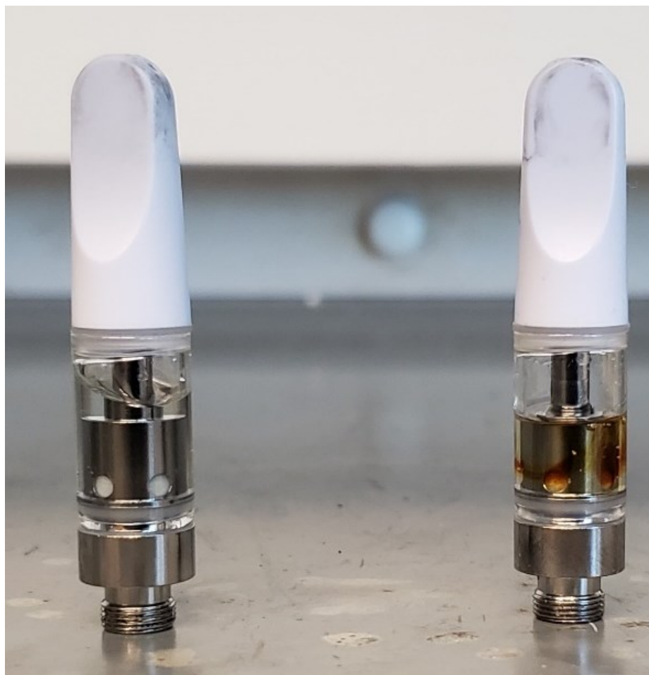
Figure S3.3. Cartridges heated at 176 and 356 °C. Visible degradation and discoloration could be seen in the cartridge heated at 356 °C (right) versus the cartridge heated at 176 °C (left) after 13 cycles of 4s battery activation during temperature measurements.
