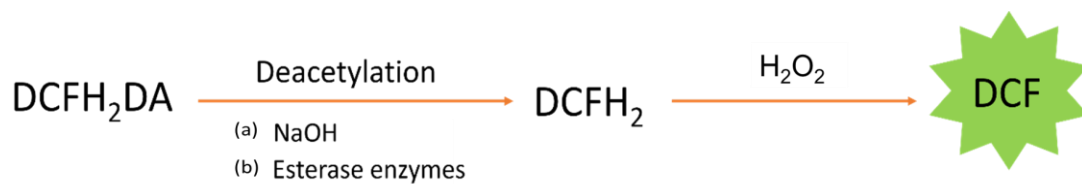
Figure S2.8. DCF reaction scheme; non-fluorescent 2',7'-Dichlorofluorescein diacetate can be hydrolyzed with (a) NaOH for acellular systems or (b) cellular esterases for cellular systems, then oxidized by ROS to form the fluorescent DCF product.
