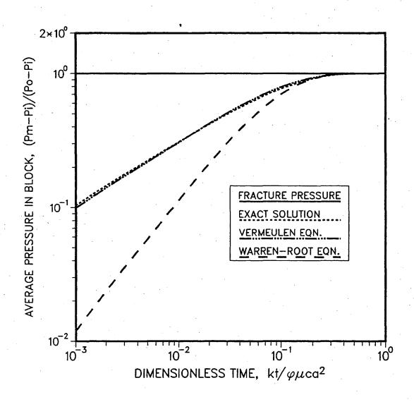
Fig. 1. Average matrix pressure in a spherical block that is subjected to a stepfunction increase in pressure at its outer boundary.
