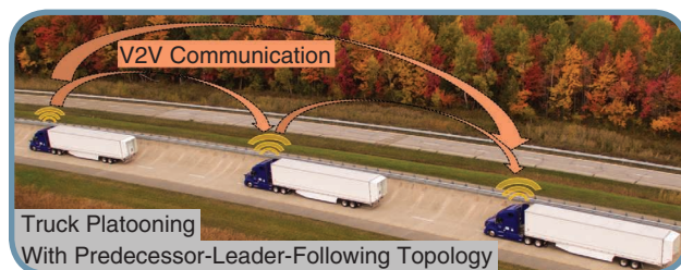
FIG 3 CACC for heavy-duty trucks: “Truck platooning”.
