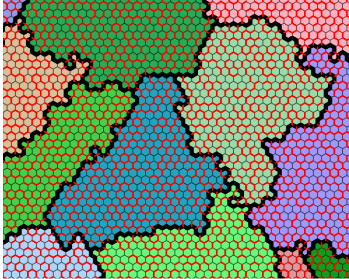
Figure 3.5: A close-up view of an Eden cluster growth model result. The red lines indicate ‘twin’ boundaries; black lines are ‘TRD’ boundaries. Other boundaries are shown in gray. The background color distinguishes each TRD.
