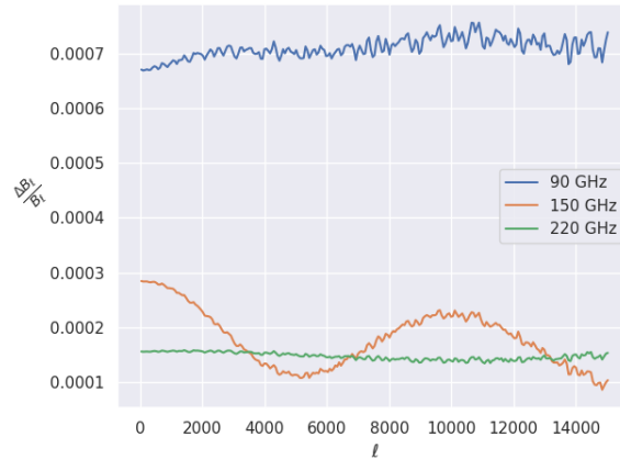
Figure 4.12: The fractional error on the beam recovered from a simulation. The dominant effect is a multiplicative scaling, which is degenerate with absolute calibration (and much smaller than our uncertainty on the absolute calibration). The variation with multipole \ell is \mathcal{O}(10^{-4}) , and much smaller than the beam uncertainties.
