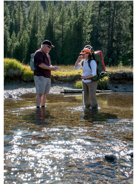
Erin Bray takes field measurements of streambed hydraulic conductivity using a backpack permeameter in the upper San Joaquin River, CA with geomorphologist Mitchell Swanson. Jennifer Natali, PhD Candidate at UC Berkeley
