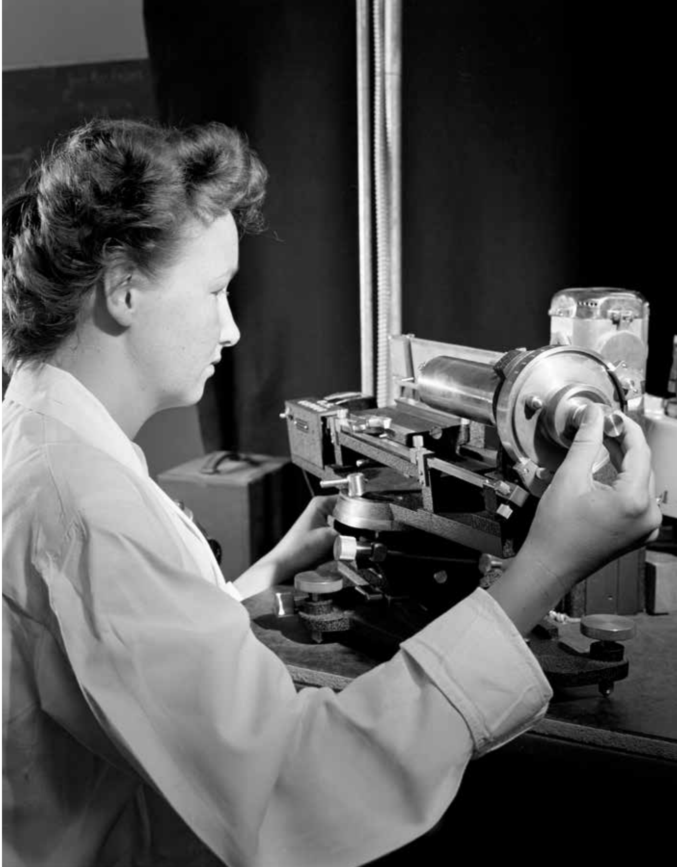
1949 › Carol H. Dauben in her lab in 318 Lewis Hall demonstrates the use of a Unicam X-ray refraction camera. Dauben (M.S. '47, Physics) was the wife of chemist William Dauben. They met after he arrived on the faculty, and she was a student. Dauben and David Templeton co-authored a number of research papers in crystallography research.
