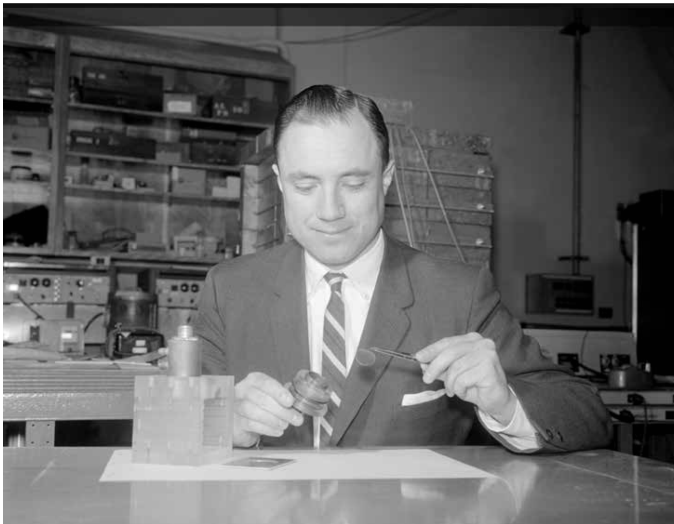
1963 › Professor of Chemistry Samuel Markowitz is the inventor of a trace analysis technique that demonstrates a Helium-3 activation. In the photo, thin aluminum foil containing one ten-trillionth of an ounce of oxygen molecules is removed from a target holder.
