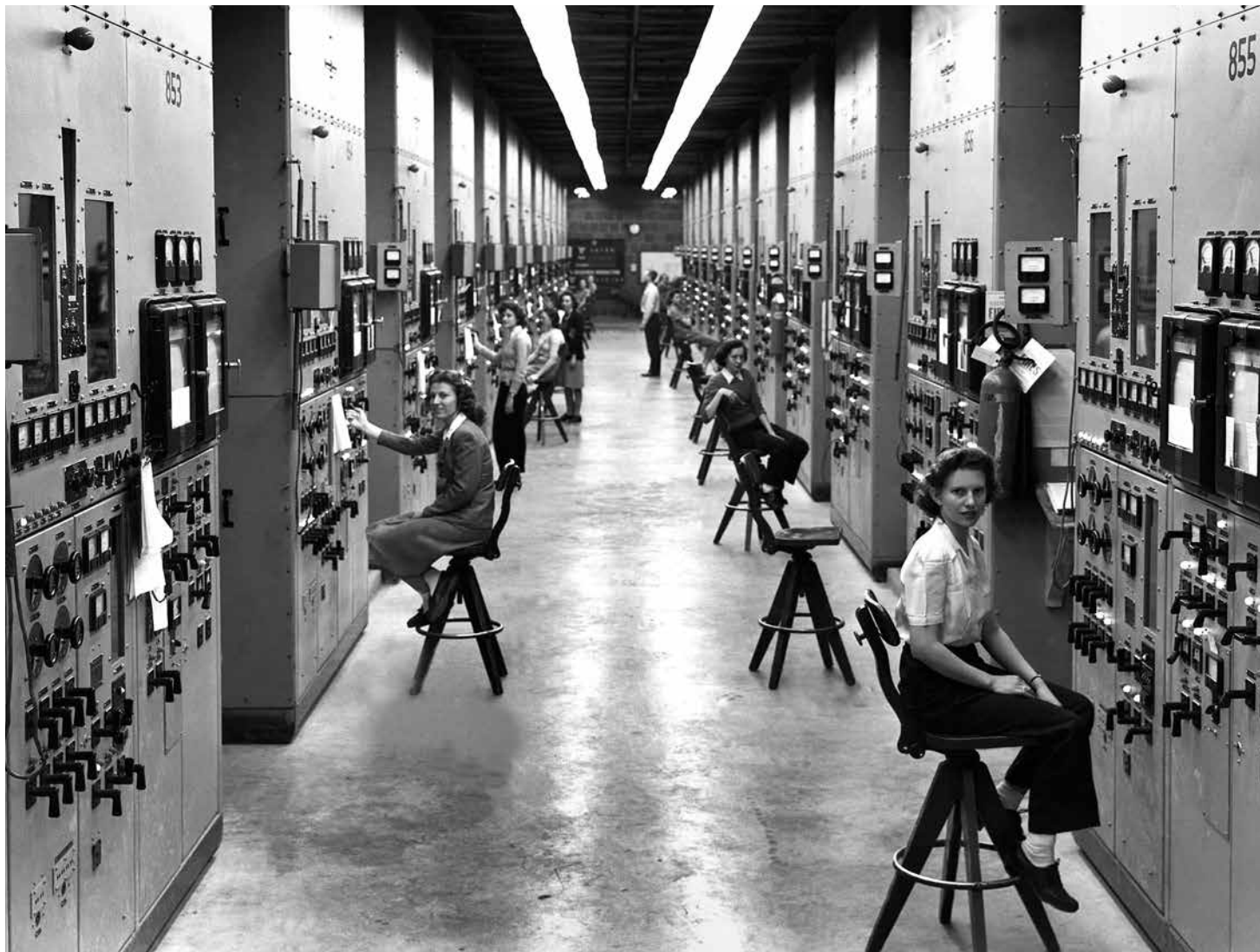
1944 > Y-12 Calutron Operators monitored components of the machines used to separate isotopes of uranium for the manufacture of the Hiroshima atomic bomb. Calutron operators were predominately female high school graduates who worked in shifts 24 hours a day. The women were considered more adept for the job of managing the machinery than the chemists working on site. The young women were not told what they were working on and only learned 50 years later the real nature of their work.
