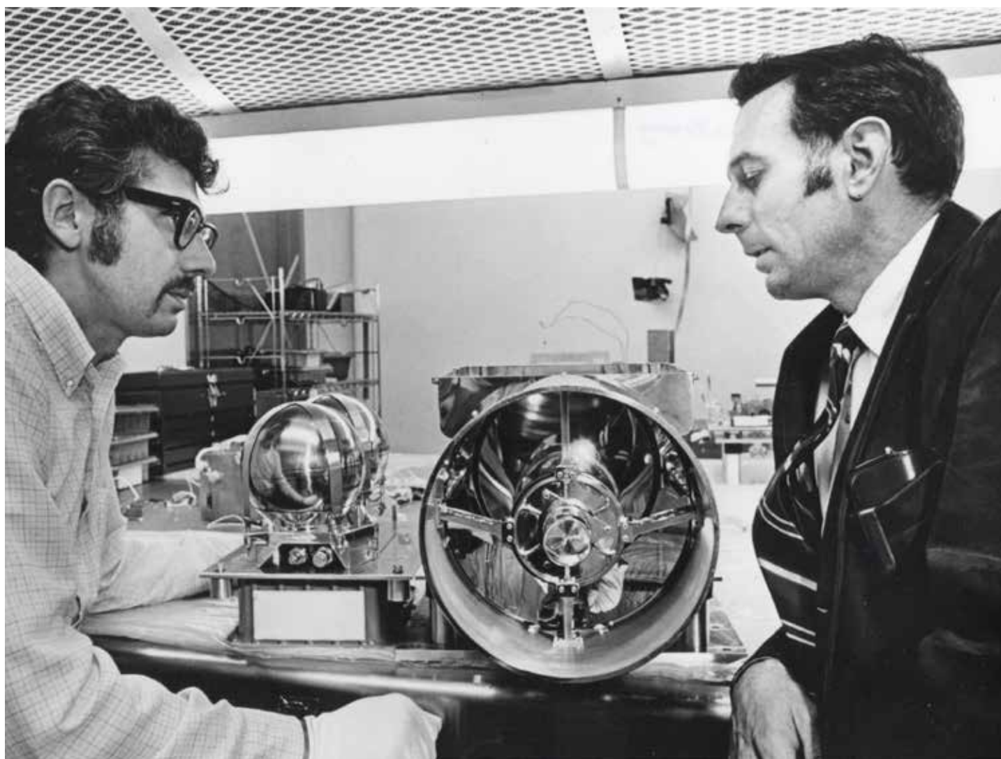
1969 › George Pimentel and Kenneth Herr review the infrared spectrometer built at UC Berkeley by the machine shop and used in the Mariner Mars 6 and 7 missions.
