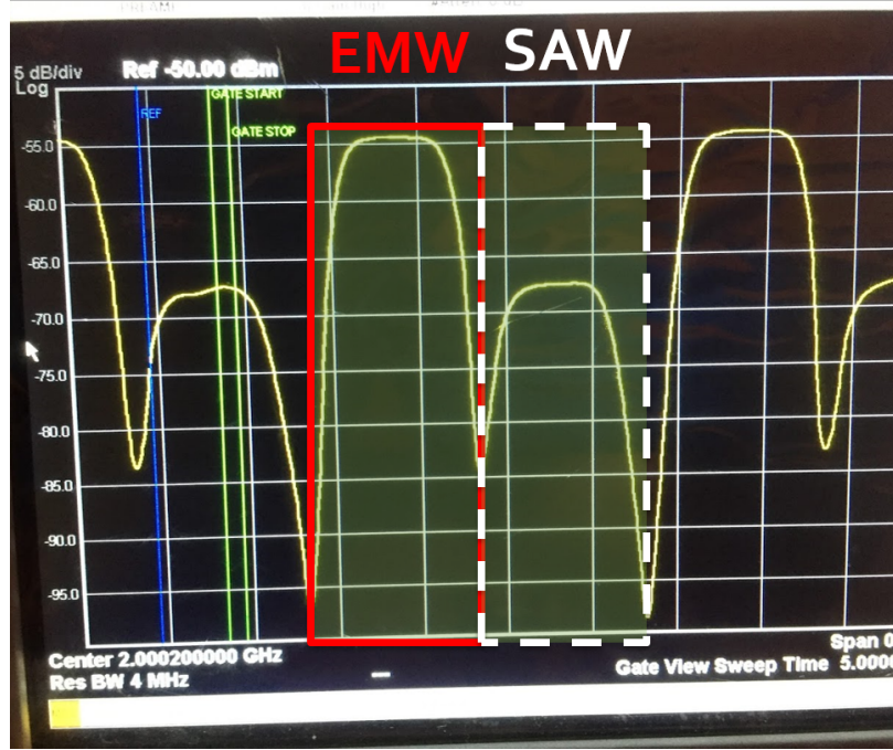
Figure 2.11: Image of spectrum analyzer screen while performing a hardware time gating measurement. The electromagnetic wave (red box) appears with a time delay of \approx 0 , while the SAW (white box) can be seen after a delay of \approx 800 ns. The pulse width is 700 ns.
