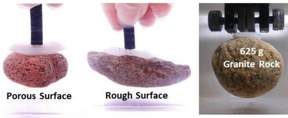
**Figure 3.7:** **A** An artificial suction disc picks up a cratered stone. **B** An artificial suction disc picks up the concave surface of a fractured granite rock. **C** An artificial suction disc lifts a 625 gram granite rock. All tests were performed and imaged underwater.
