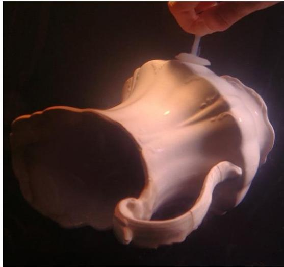
**Figure 4.1: Suction disc adhering to and lifting an example of an archaeological artifact while underwater.**
