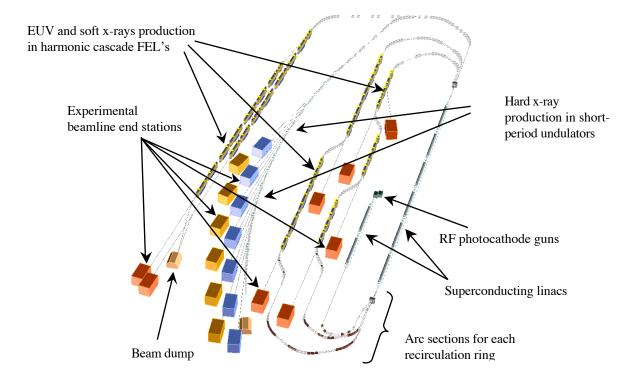
Figure 1. LUX machine layout. The machine footprint is approximately 150x50m. A capacity of approximately 20 beamlines is available, using a combination of harmonic cascade FELs and spontaneous emission in insertion devices.
