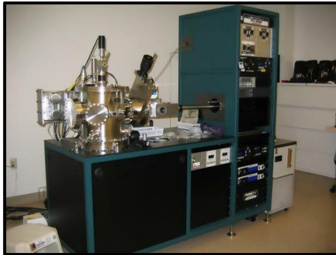
Figure 7 The AJA sputtering system used to deposit many types of thin films. The system is capable of depositing multiple materials concurrently through either manual operation or automatic programming.
