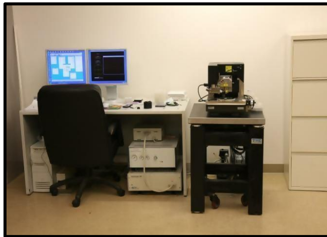
Figure 8 Atomic Force Microscope (AFM) system used for MFM and AFM measurements. This system is capable of measuring surface roughness, thicknesses, and magnetic domains of the thin films.
