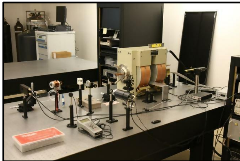
Figure 11 The system set up used in transmission mode (Faraday Effect).
