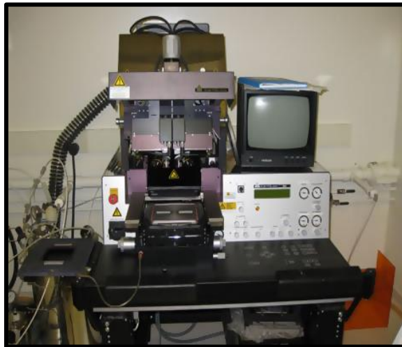
Figure 6 The Karl Suss MA6 mask aligner instrument used in the CNSE at UCR used to create patterned substrates.
