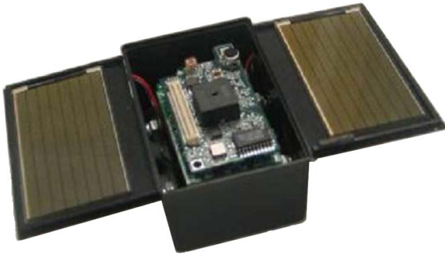
Fig. 3. Helimote, a solar harvesting sensor node.
