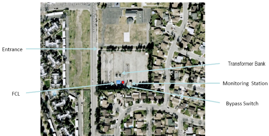
Figure 59: FCL Installation in Avanti Circuit of the Future. Shandin Substation, San Bernardino, California, March 2009.
