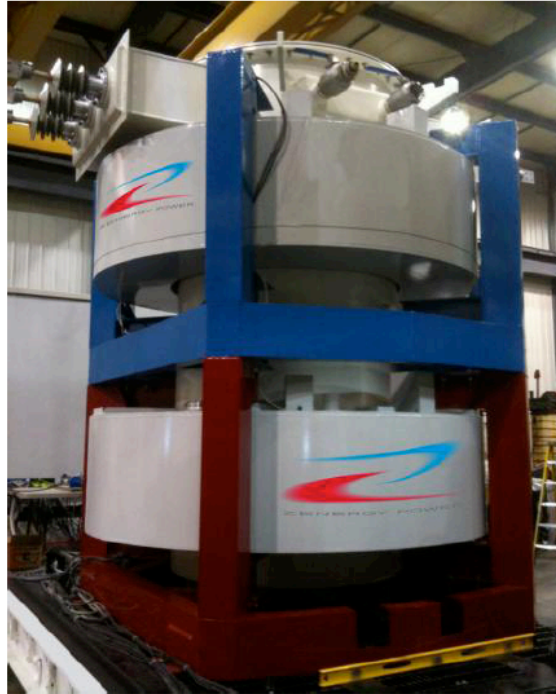
Figure 76: Three-phase distribution-level, 15kV class, Compact FCL prototype with “dry-cooled” HTS magnets surrounding an oil-filled dielectric tank with AC coils.
