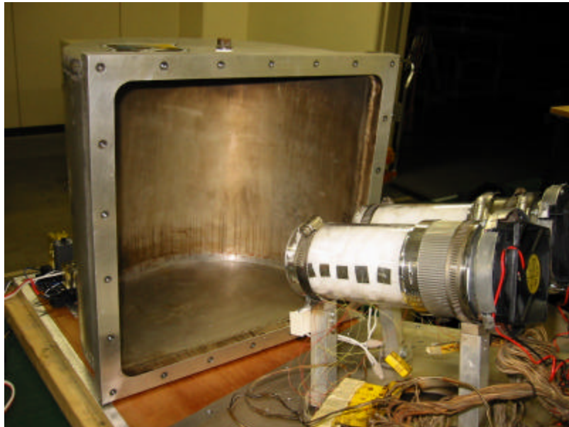
Fig. 2 Photograph of combustion chamber and two instrumented sample holders
