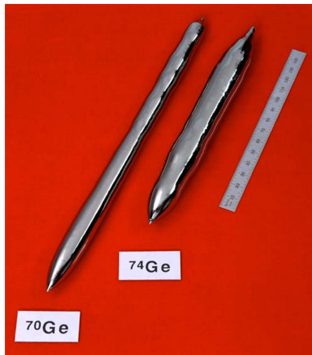
Fig. 1. Photograph of 95% enriched, ultrapure Ge single crystals. The ruler is 150 mm long.
