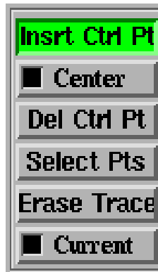
Figure 9: Trace editing controls. The trace editing button Insrt Ctrl Pts is activated, i.e. green, with the Center checkbox activated causing subsequent control points inserted to be vertically centered in the Current trace indicated in the Line # dialog box.
