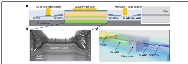
**Fig. 6 Heteroepitaxial laser integration on Si photonic platform. a** Schematic diagram of the heteroepitaxial laser integration on Si platform. **b** Cross-section TEM of full laser epi in the pockets grown on 300 mm Si from IQE. **c** Schematic of intended device configuration.
