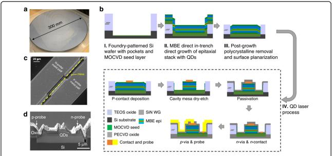
Fig. 4 Fabrication process of the in-pocket laser. a As-grown 300 mm wafer from IQE, covered with polycrystal III–V. b Simplified fabrication flow for laser fabrication, not drawn to scale. c Top-down view of an as-fabricated device. d Cross-section SEM of the as-cleaved in-pocket laser.
