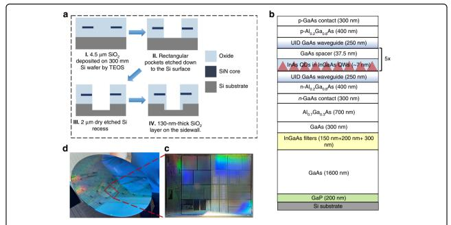
Fig. 1 Template preparation and proposed laser stack. a Schematic diagram of the pattern formation process before III–V deposition. b Simplified III–V laser stack. c The diced coupon from the as-patterned 300 mm Si wafer for growth condition investigation. d As-patterned 300 mm Si wafer.
