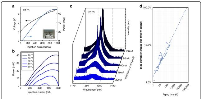
Fig. 5 Laser measurement results. a Room-temperature LIV of the device with the highest output power. Inset shows the probe needles on a cleaved laser bar. b Temperature-dependent LIV shows lasing up to 60 °C. c Lasing spectrum as a function of injection current at room temperature. d Aging results for the in-pocket laser at 35 °C.
