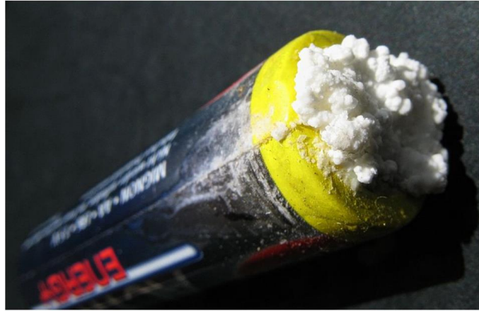
Figure 6.1. Leaked alkaline battery illustrating the formation of KOH crystals[143].
